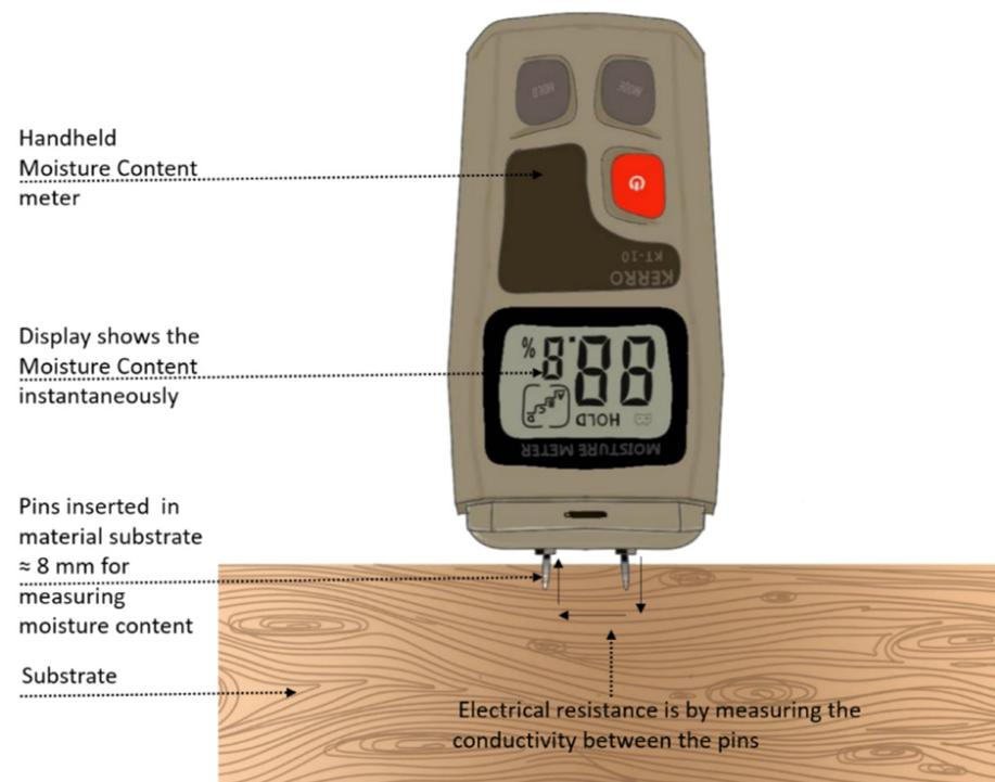
**Figure 3.** Measurement of a surface's moisture content. (Source: authors).
