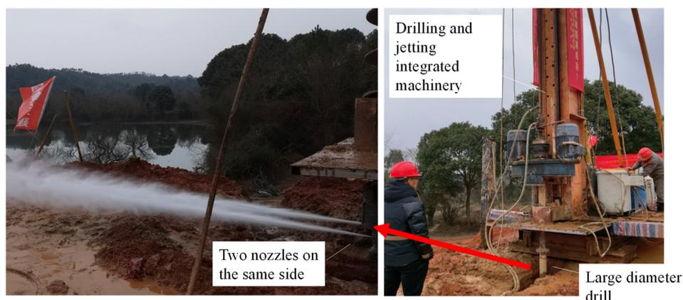
**Figure 2.** The self-developed ipsilateral, multi-nozzle, high-pressure jet bit and ground jet test.
