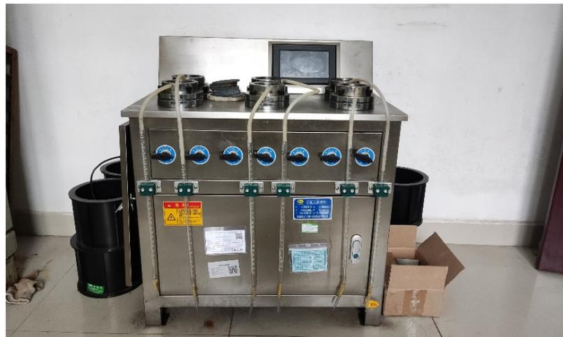
**Figure 4.** SS-2.5 cement soil permeameter.
