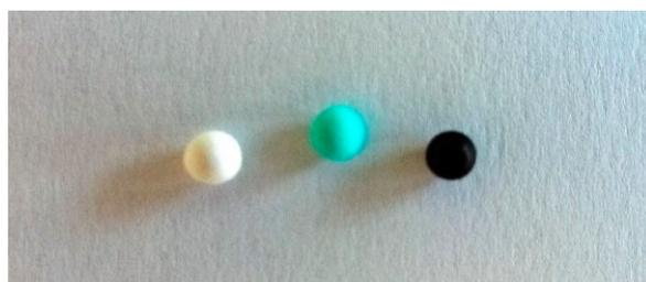
Figure 2. Different stages of CuO preparation: only Al<sub>2</sub>O<sub>3</sub> (white), Al<sub>2</sub>O<sub>3</sub> with adsorbed copper salt (blue), and Al<sub>2</sub>O<sub>3</sub> with CuO (black).
