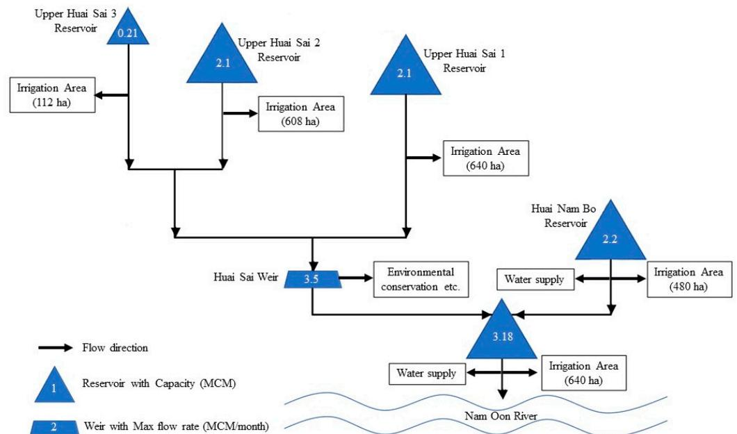
Figure 2. Schematic Diagram of the Multi-Reservoir System in Thailand.
