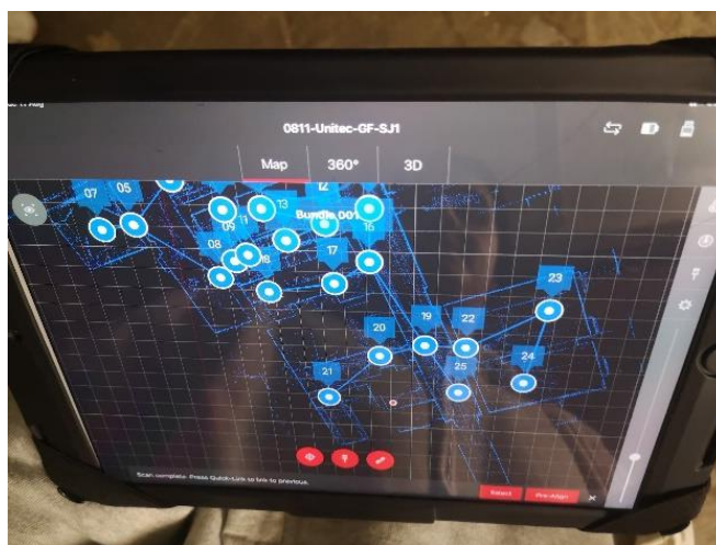
Figure 2. Linking scans on Leica Cyclone on iPad during scanning of Building One.
