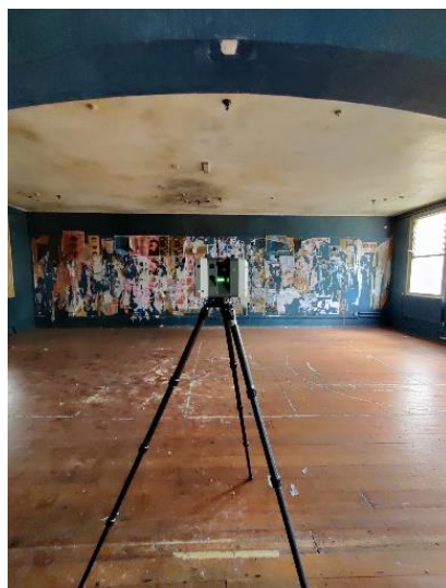
Figure 1. Leica RTC360 during scanning of Building One.
