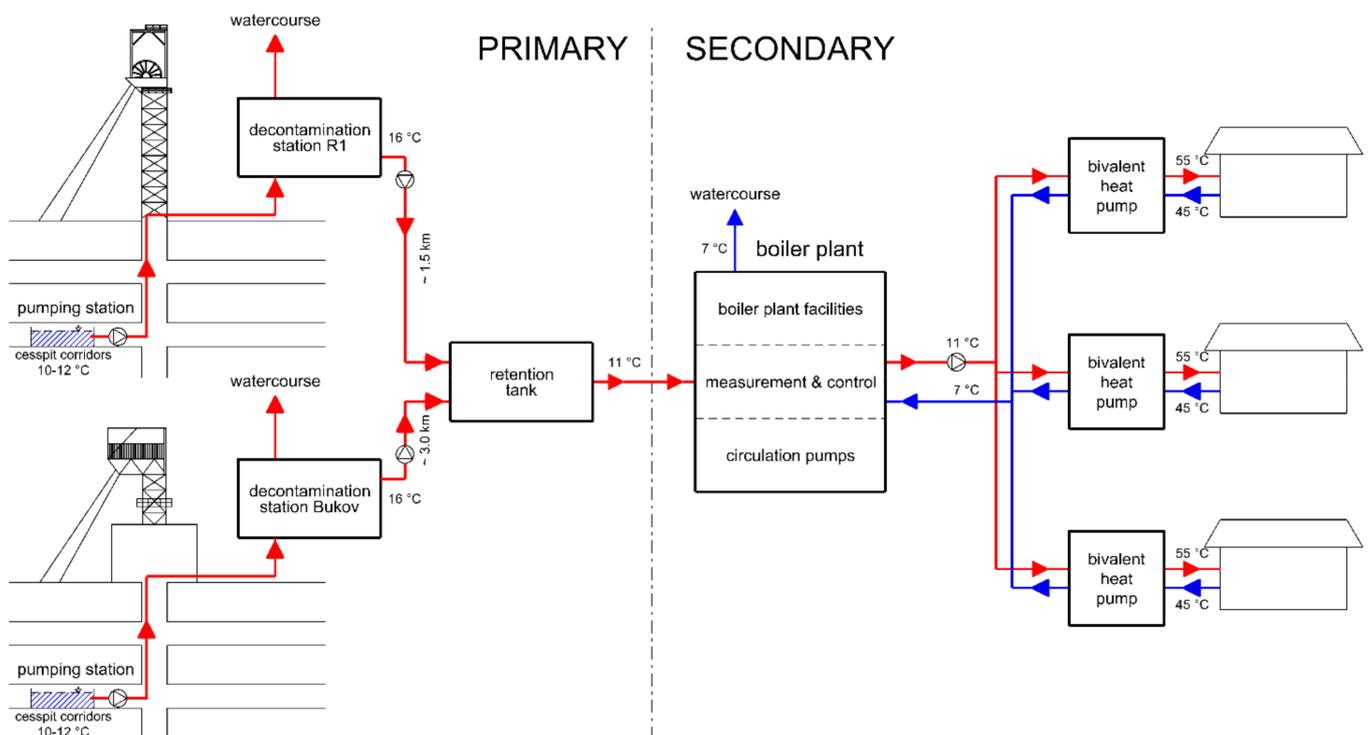
**Figure 9.** Schematic representation of Option 3 heat recovery of decontaminated water.
