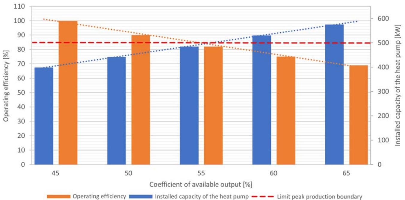
Figure 7. Comparison of heat production of Option 2 with the limit requirement for the heat pump output.
