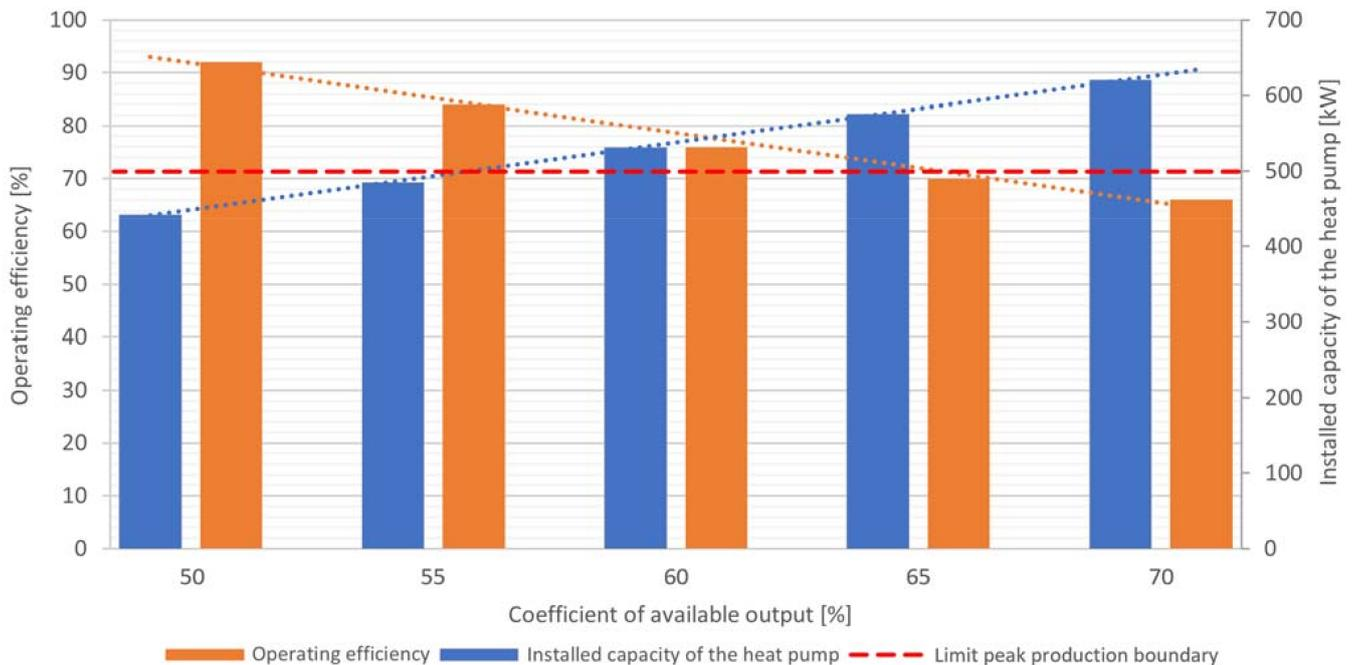
Figure 5. Comparison of heat production of Option 1 with the limit requirement for the heat pump output indicated.
