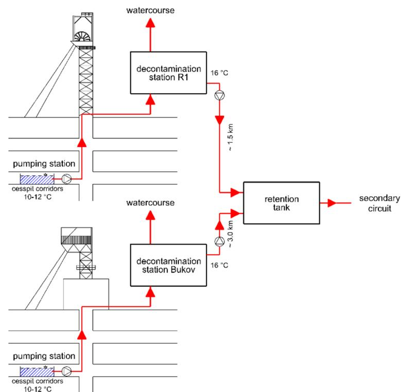
Figure 3. Schematic representation of the primary heat recovery circuit for decontaminated water.
