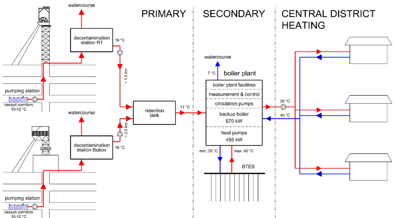
Figure 6. Schematic representation of Option 2 heat recovery of decontaminated water.
