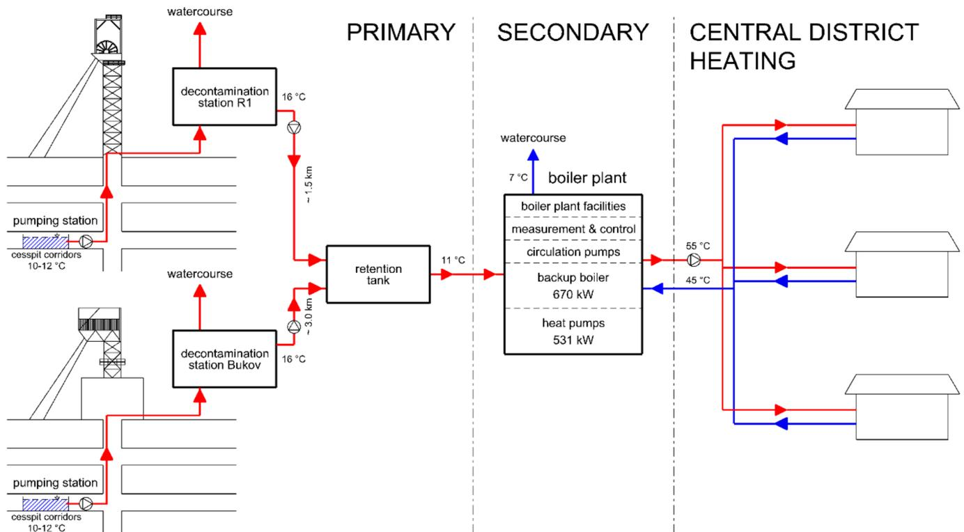
Figure 4. Schematic representation of Option 1 heat recovery of decontaminated water.
