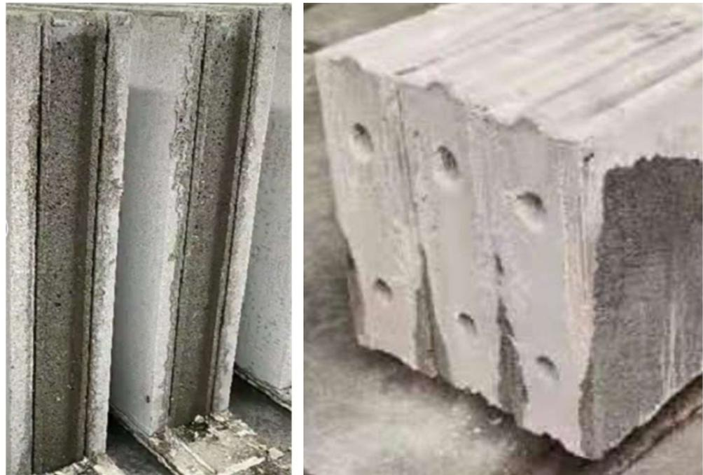
**Figure 1.** Composite wallboard with foamed ceramic board and foamed concrete.
