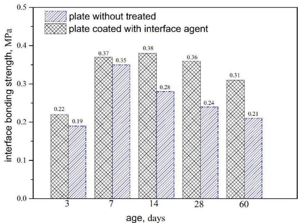
**Figure 4.** Effect of treatment of the foamed ceramic board on bonding strength of the composite wallboard with different ages.
