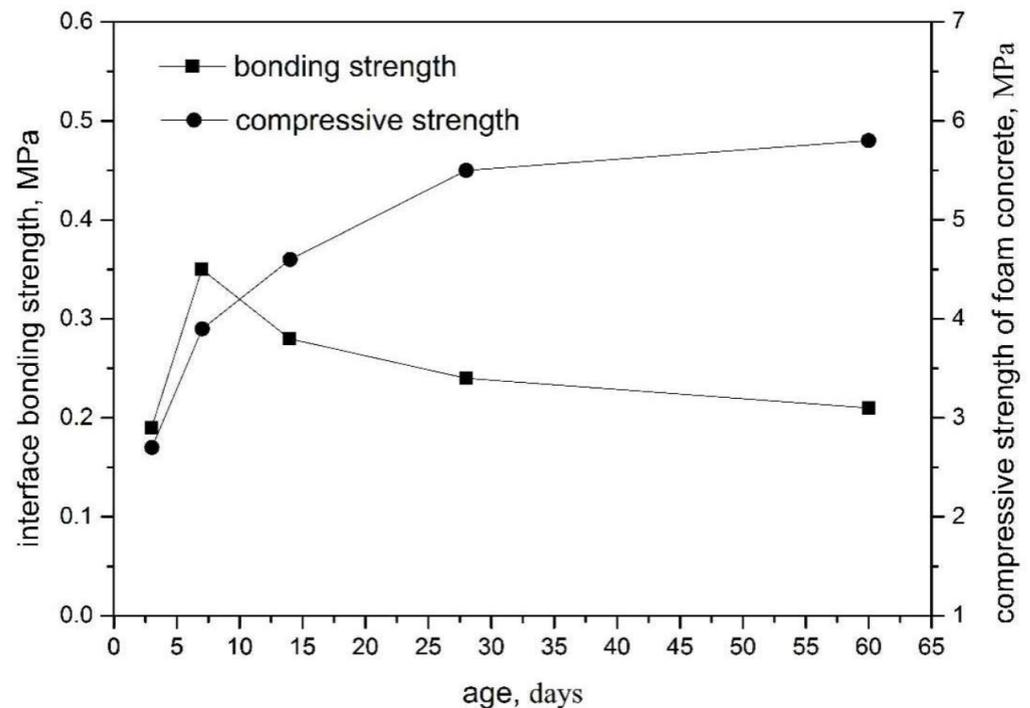
**Figure 2.** Effect of foam concrete age on the interface bonding strength of composite wallboard and the compressive strength of foam concrete.
