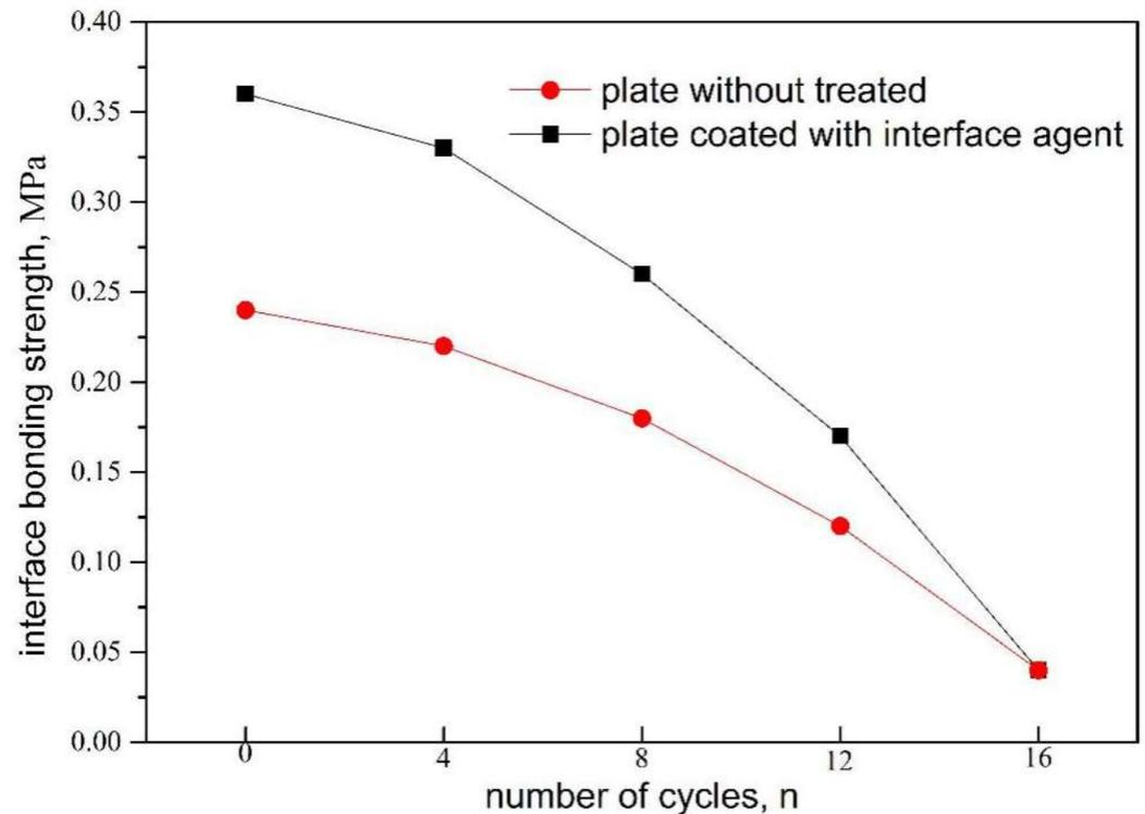
Figure 5. Effect of freeze–thaw cycles on interface bonding strength.
