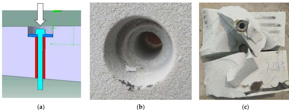
**Figure 8.** Schematic diagram of single-point loading and failure characteristics of foamed ceramic plates: (a) single-point loading diagram; (b) failure characteristics of non-adhesive sleeve placed in long hole; (c) failure of plastic sleeve placed in long hole feature.
