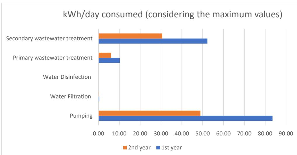
**Figure 4.** Energy consumption in the winery, considering the maximum values referred to in the literature, for each process.
