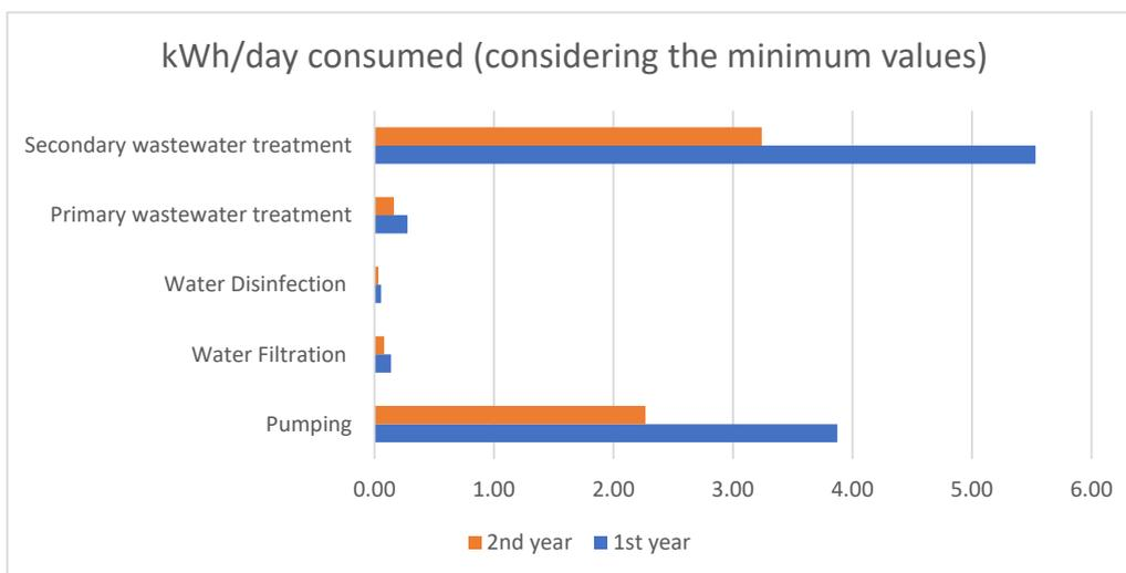
**Figure 3.** Energy consumption in the winery, considering the minimum values referred to in the literature, for each process.
