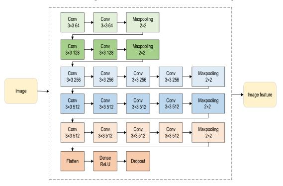
Figure 5. The image feature extraction model structure diagram.
