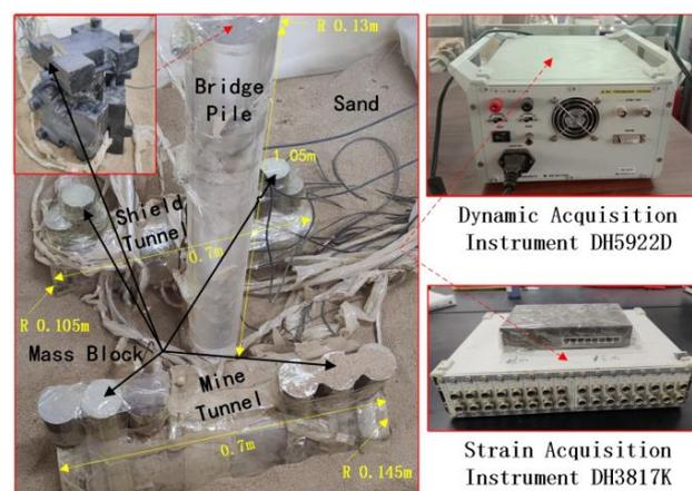
**Figure 4.** Model, counterweight, and acquisition instrument.
