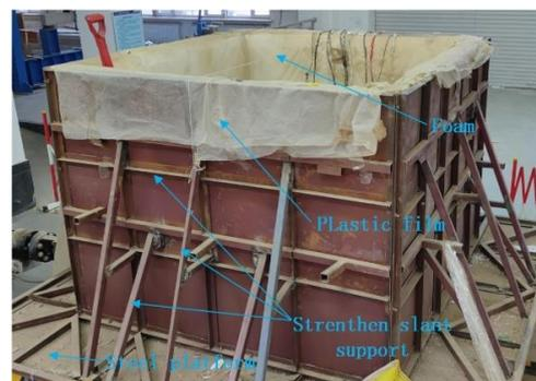
**Figure 3.** Model soil container.
