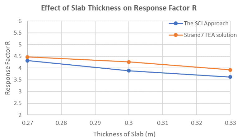
Figure 15. The Effect of the slab thickness on Response Factor R.
