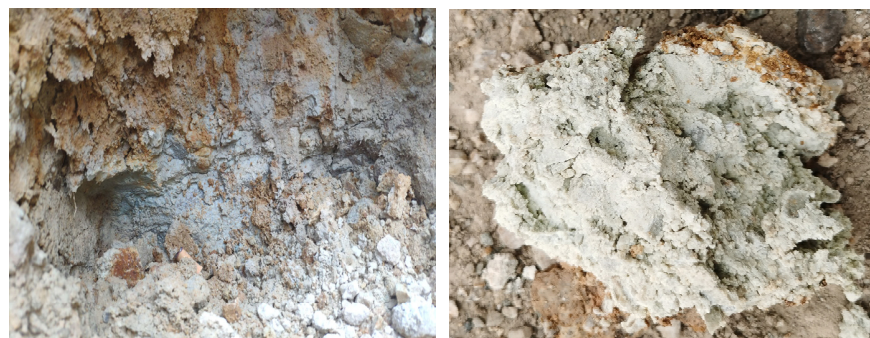
Figure 7. Grayish white–white silty clay revealed by borehole drilling results at the bottom of the toppling-falling zone.
