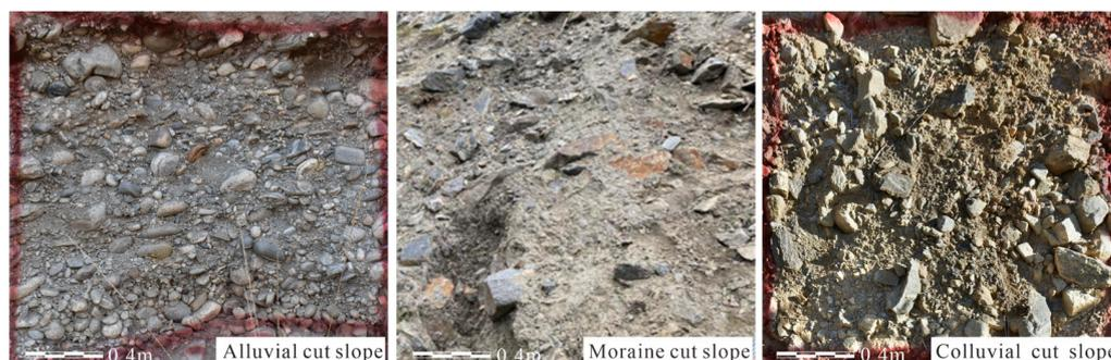
**Figure 4.** Material composition characteristics of alluvial deposits, moraine deposits, and colluvial deposits cut slopes along the Pai-Mo road.
