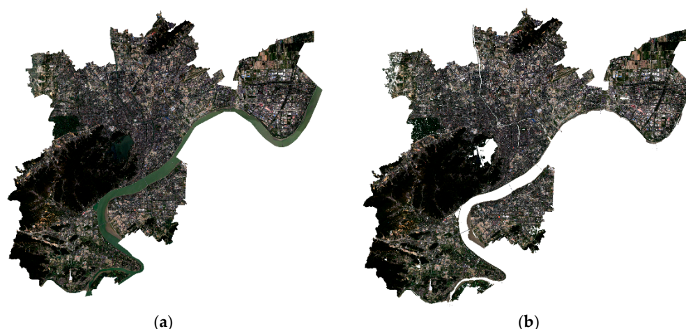
Figure 3. Masking of water bodies based on NDWI (main built-up area in Hangzhou): (a) before masking; (b) after masking.
