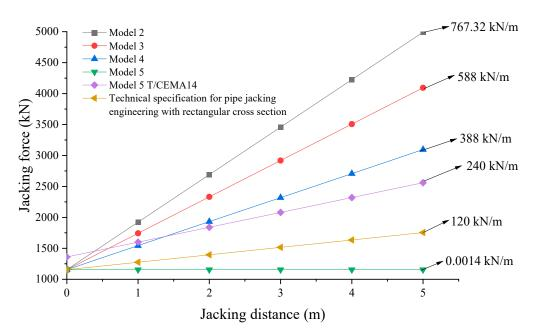
Figure 10. Partially enlarged detail of jacking force prediction with distance under different models.
