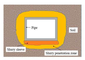
Figure 5. Pipe–slurry interaction at the bottom.
