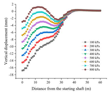
**Figure 15.** Vertical displacements of ground surface above the jacking axis under different grouting pressures when the tunneling distance is 30 m.
