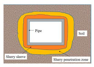
Figure 8. Full contact pipe-slurry interaction.
