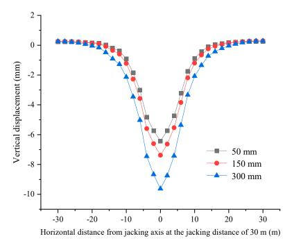
**Figure 12.** Vertical displacements of ground surface at the jacking distance of 30 m (the cross-section y = 30 m) under different slurry sleeve thicknesses after finishing jacking.
