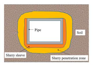
Figure 7. Pipe–slurry interaction at the bottom and both sides.
