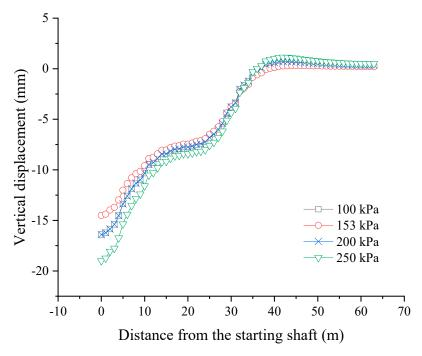
**Figure 17.** Vertical displacement of ground surface above the jacking axis under different earth chamber pressures when the tunneling distance is 30 m.
