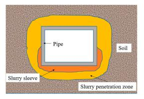
Figure 6. Pipe–slurry interaction at the bottom and 1/2 of both sides.
