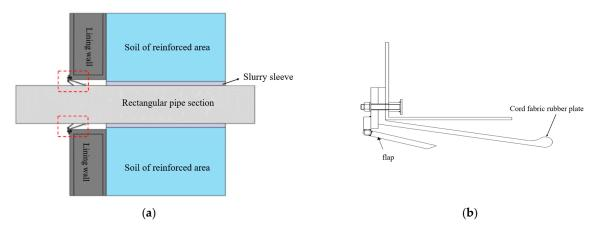
**Figure 18.** Installing waterproof rubber curtain for the tunnel portal: (a) longitudinal section of the waterproof device; (b) details of the waterproof device.
