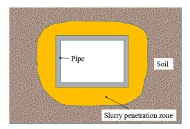
Figure 3. Full pipe-soil contact model.
