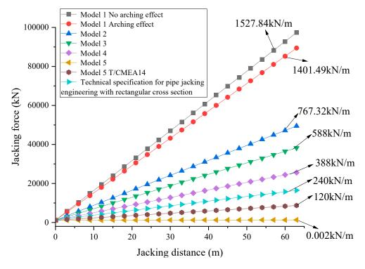
Figure 9. Jacking force prediction with distance under different models.
