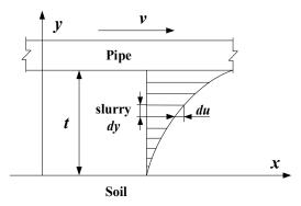
Figure 2. Schematic diagram of interaction between pipe and slurry.
