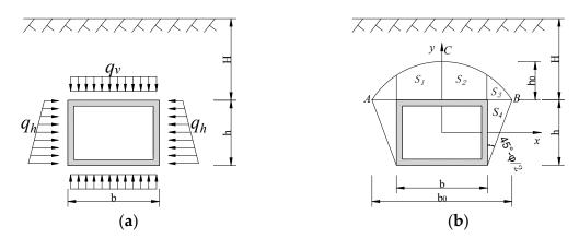
Figure 4. Stress diagram of full pipe–soil contact: (a) no arching effect; (b) arching effect.
