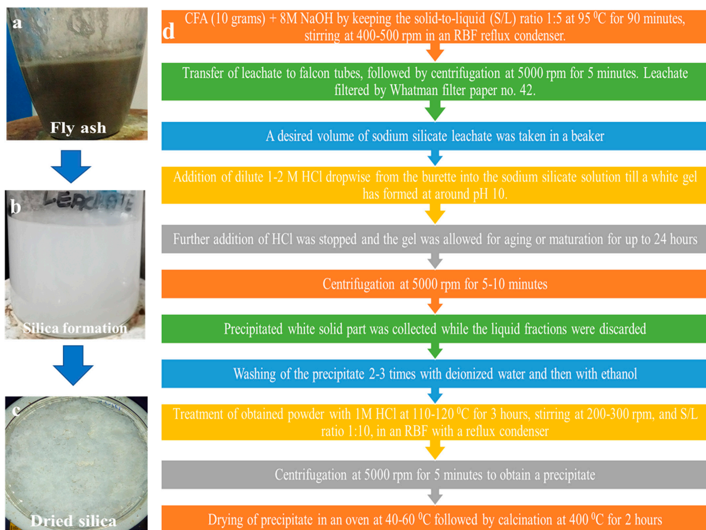
Figure 1. (a–d) Steps involved in the synthesis of nanosilica from coal fly ash.
