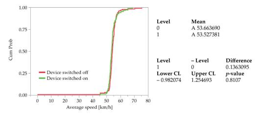
Figure 4. Cumulative representation of average speeds in an hour on road D1 in Mirkovec.
