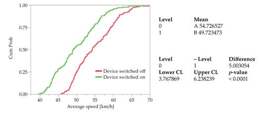
Figure 3. Cumulative representation of average speeds in an hour on road D28 in Severin.
