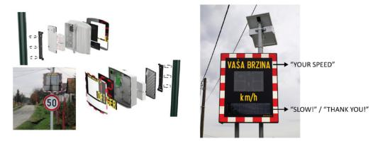
Figure 1. Speed display radar—example.
