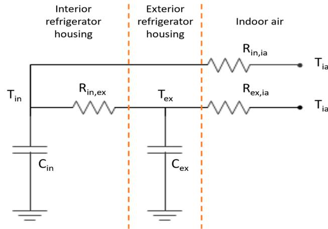
**Figure 2.** RC model for the refrigerator, freezer, and electric water heater.
