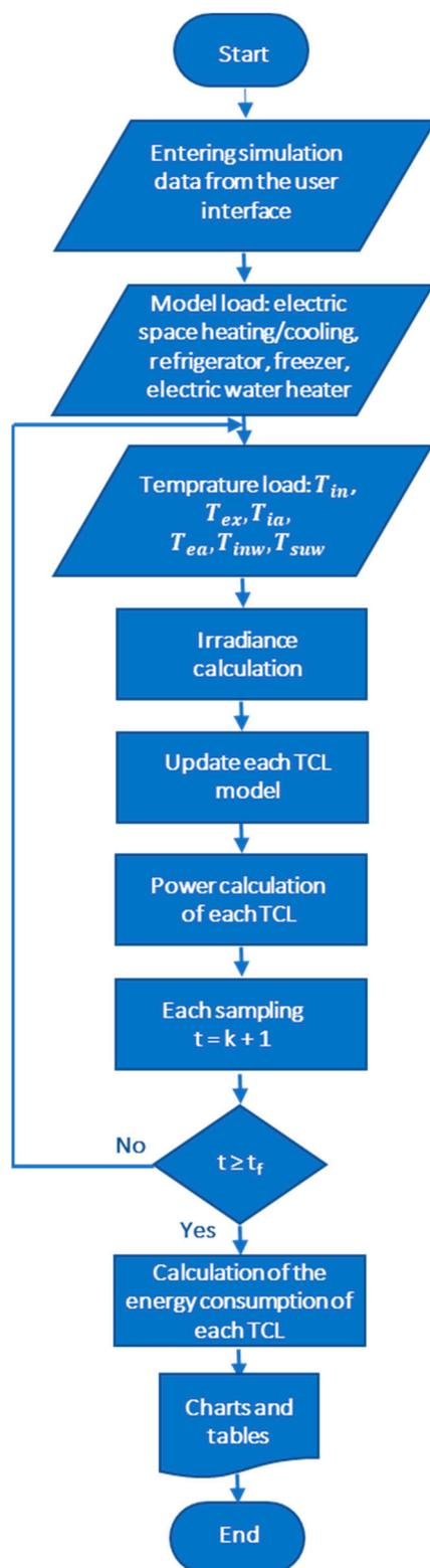
Figure 4. Flow chart of the developed SBET-TCLs.
