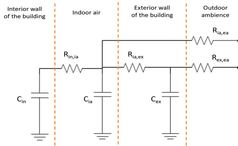
**Figure 1.** RC model for electric room heating/cooling.
