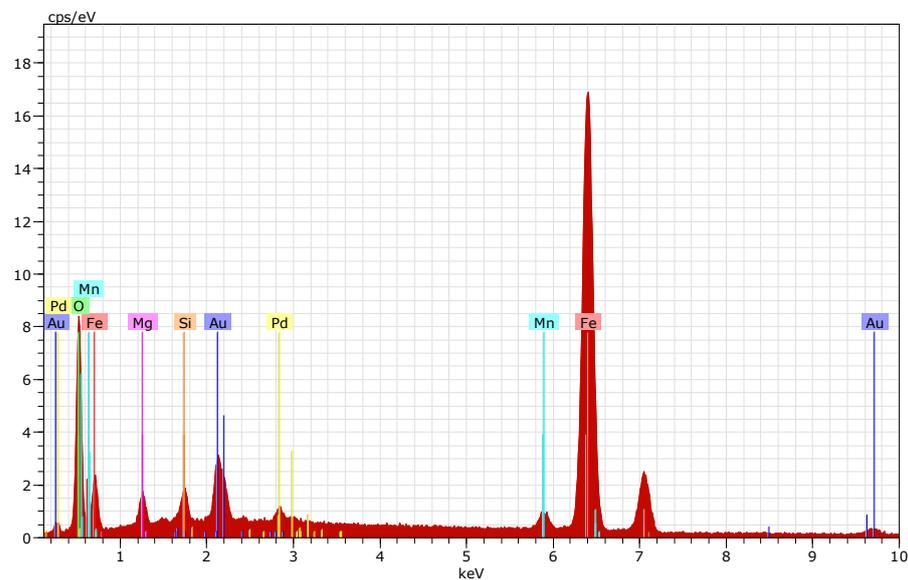
**Figure 6.** Elemental composition—quantitative analysis test no. 1.
