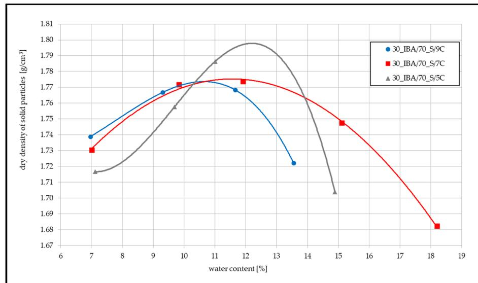
Figure 10. Water content and dry densities of solid particles for 30\_IBA/70\_S mixtures.
