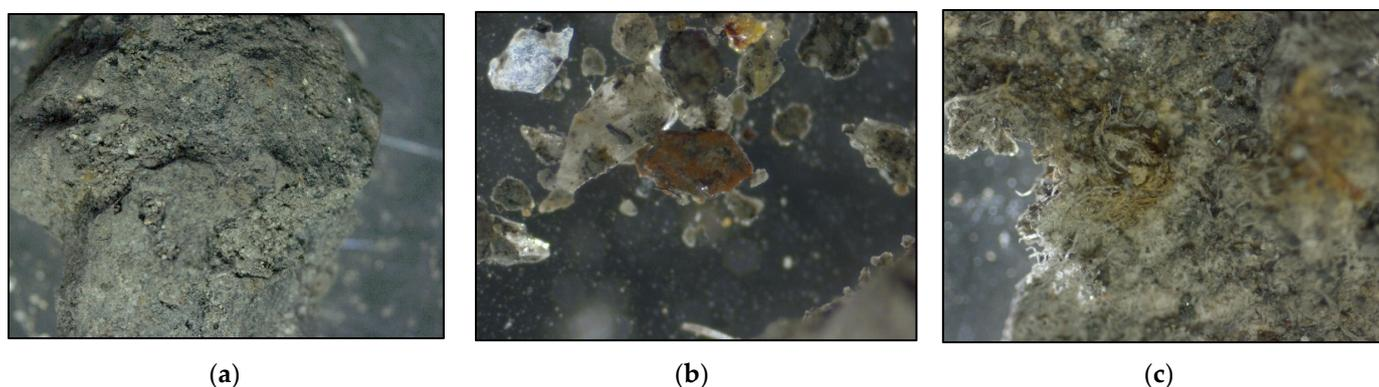
**Figure 2.** IBA binocular analysis: (a) ceramics, (b) glass, (c) fibrous material.
