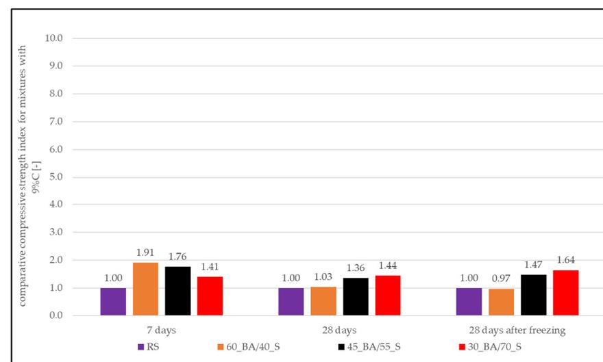
Figure 15. The comparative compressive strength index with 9% of cement.
