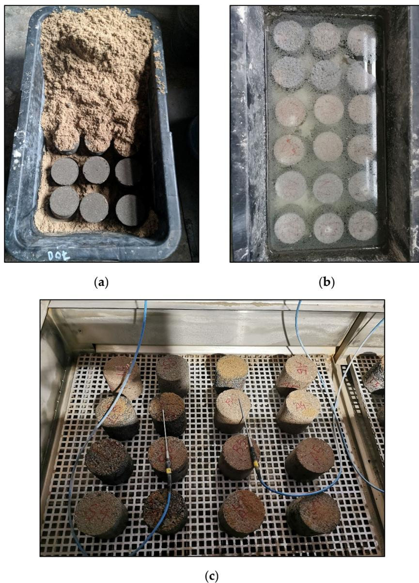
**Figure 3.** Specimen care of samples: (a) merged in wet sand, (b) fully submerged in water, (c) during the freezing cycle.
