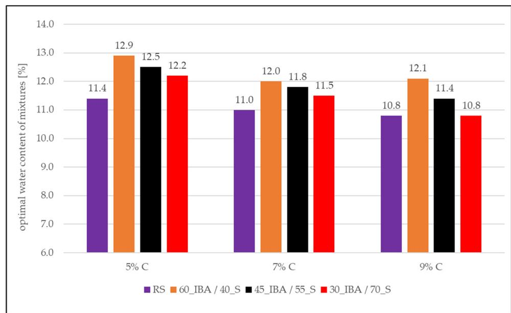
**Figure 11.** Summary of the optimal water content of analyzed mixtures depending on the amount of cement.
