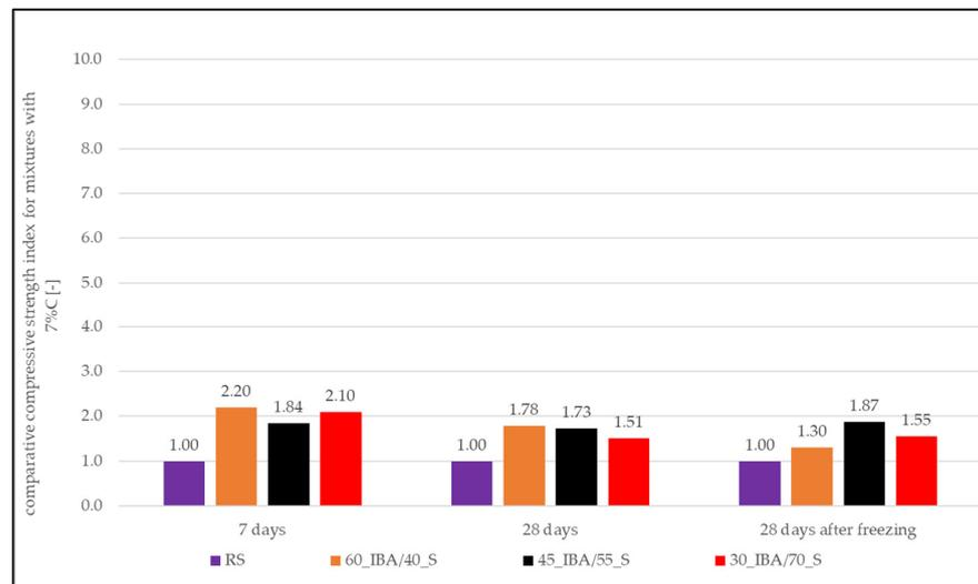
Figure 14. The comparative compressive strength index with 7% of cement.
