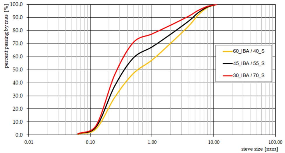
Figure 9. Granular structure curves of analyzed mixtures of IBA and sand 0/2.
