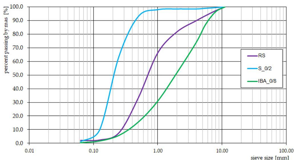
Figure 4. Granular structure curve of analyzed materials.
