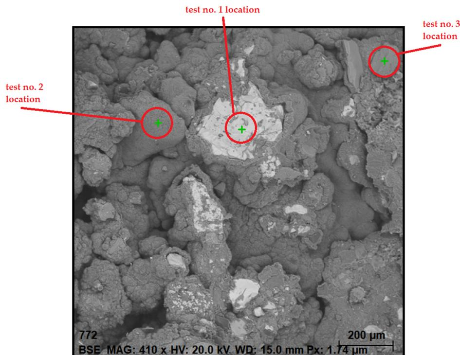
Figure 5. SEM view using EDX analysis, with three location of chemical composition tests.
