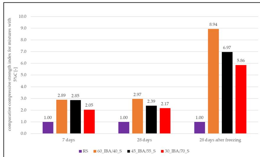
Figure 13. The comparative compressive strength index with 5% of cement.
