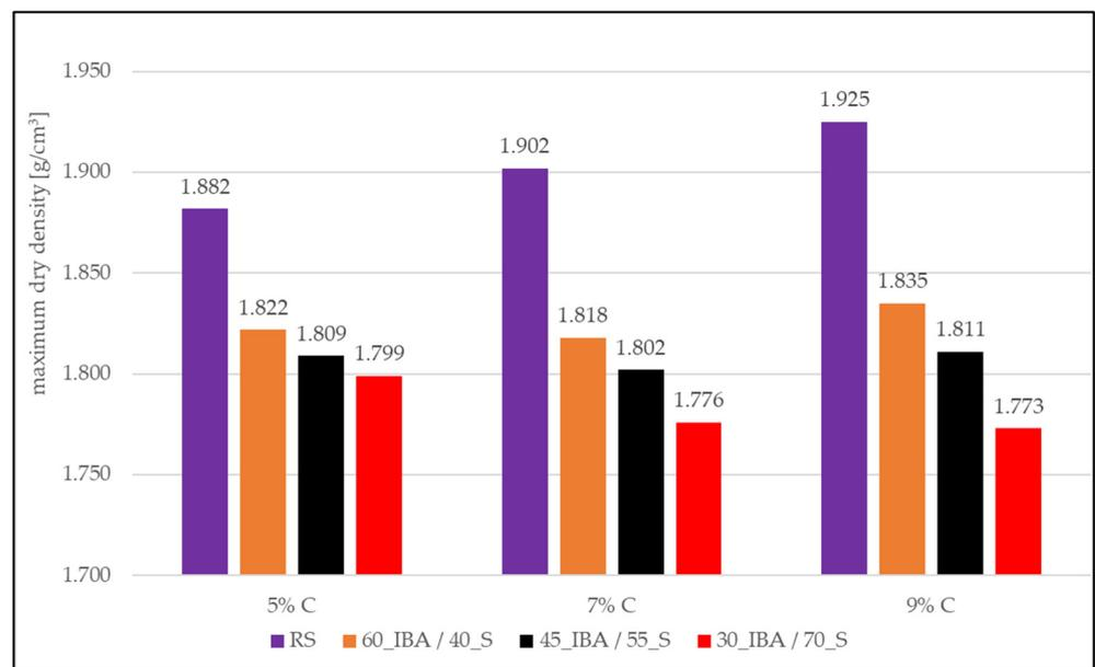
**Figure 12.** Summary of maximum dry density of solid particles of analyzed mixtures depending on the amount of cement.
