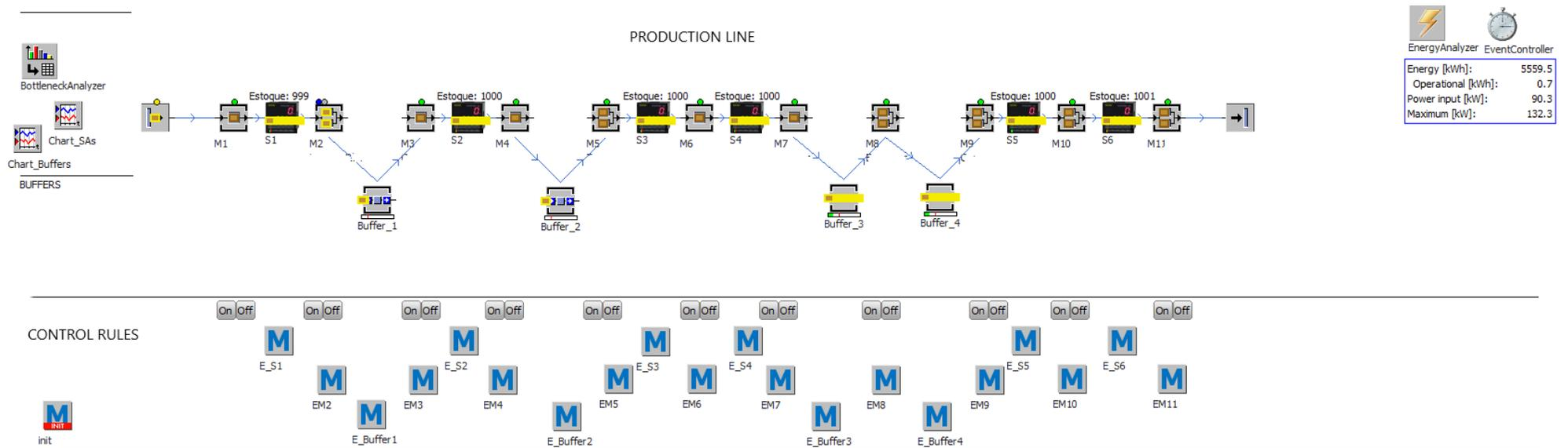
Figure 2. The flowshop process—the digital manufacturing simulation model.
