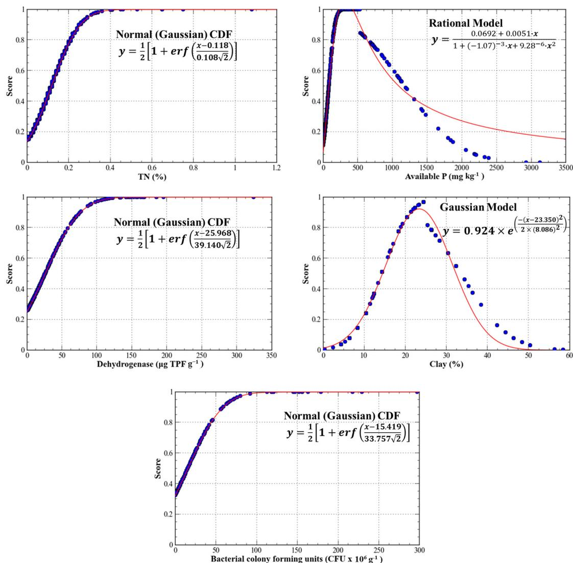
**Figure 2.** The non-linear scoring function curves of the selected five soil health indicators: total nitrogen (TN), clay content, dehydrogenase activity, available P, and bacterial CFU. Lines and circles are fitted model curves and measured soil data, respectively.
