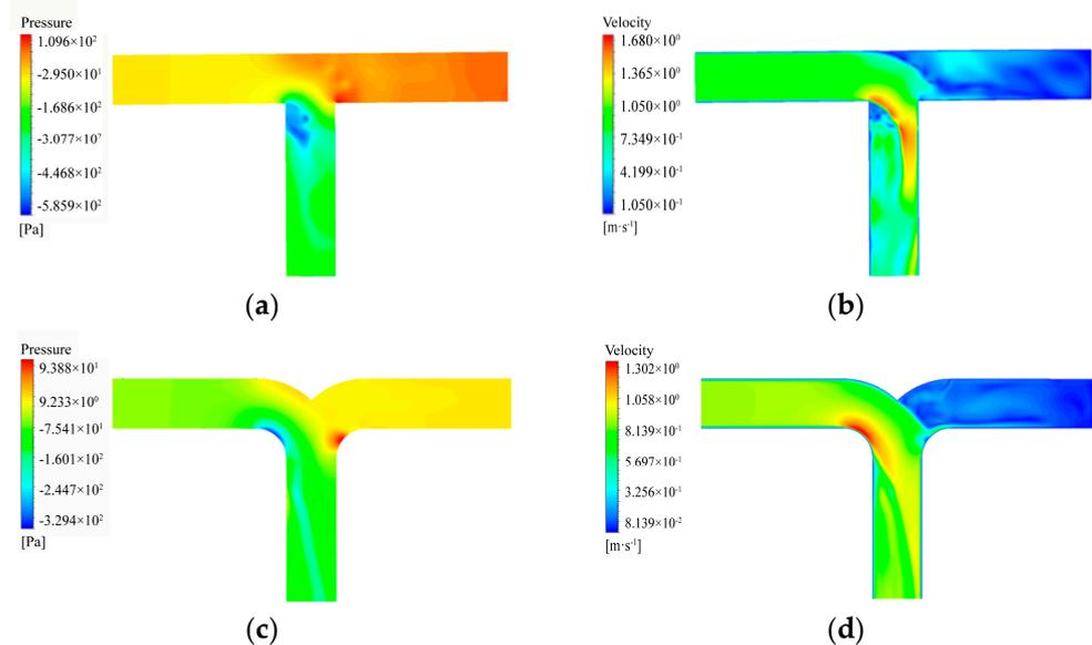
**Figure 8.** Static pressure (a,c) and velocity cloud (b,d) diagrams for conditions 4 and 8, respectively.
