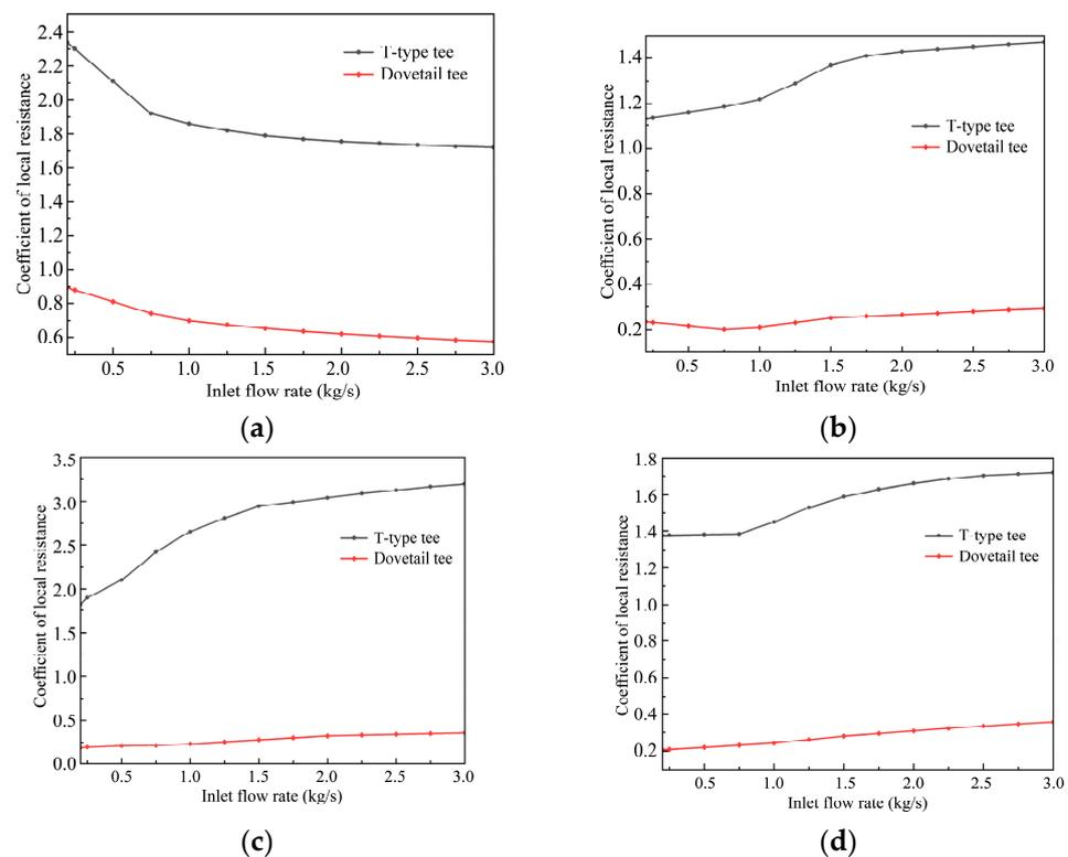
**Figure 9.** Comparisons of the local resistance coefficients for two shapes of tee: (a) conditions 1 and 5; (b) conditions 2 and 6; (c) conditions 3 and 7; (d) conditions 4 and 8.
