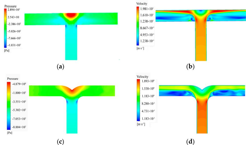
**Figure 5.** Static pressure (a,c) and velocity cloud (b,d) diagrams for conditions 1 and 5, respectively.
