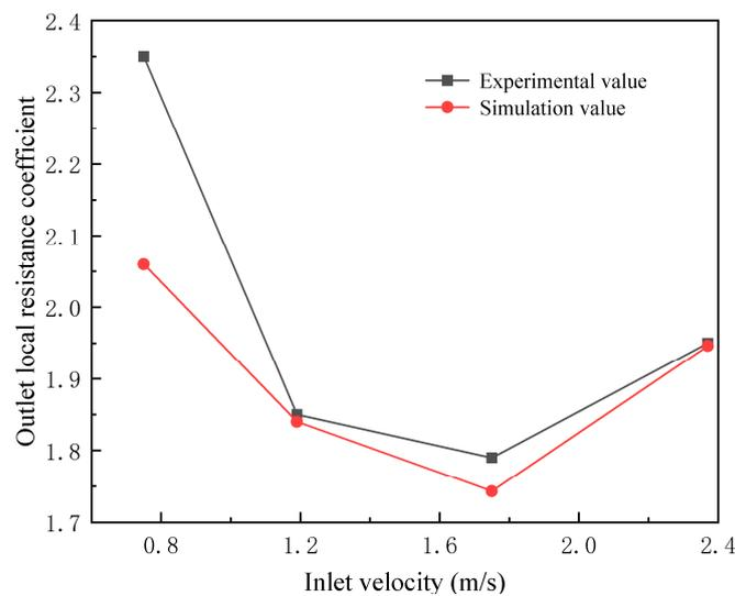
**Figure 4.** T-type tee data comparison chart.
