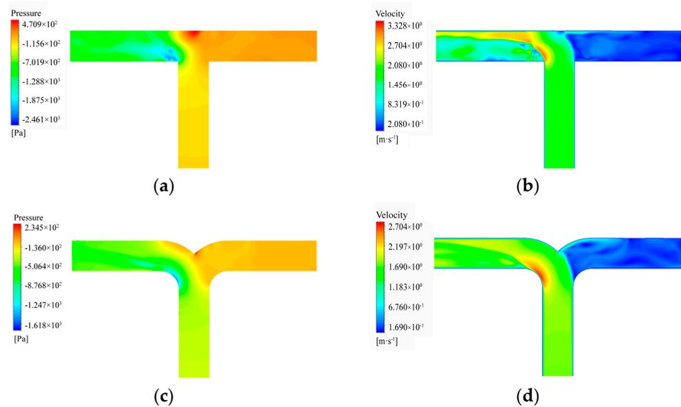
**Figure 6.** Static pressure (a,c) and velocity cloud (b,d) diagrams for conditions 2 and 6, respectively.
