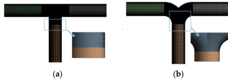
**Figure 2.** Meshes of two types of tees: (a) T-type tee; (b) dovetail tee.
