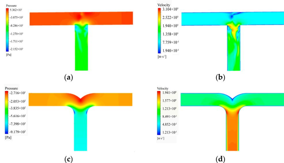
**Figure 7.** Static pressure (a,c) and velocity cloud (b,d) diagrams for conditions 3 and 7, respectively.
