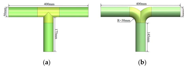
**Figure 1.** Model diagram of two types of tees: (a) T-type tee; (b) dovetail tee.
