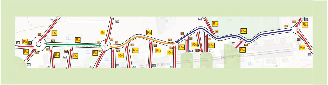
**Figure 5.** The road layout around the University of Calabria features  $R_i$  to mark 21 potential sensor locations, with  $u_i$  and  $y_i$  representing the vehicles entering and exiting the  $i$ th link, respectively.
