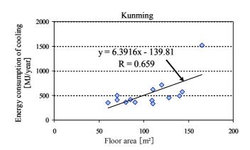
Figure 4. Correlation between consumptions of cooling and floor area.
