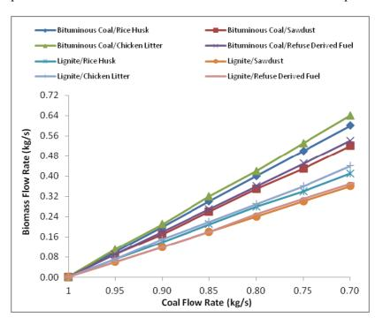
Figure 2. Comparison of coal and biomass flow rates based on a fixed heat input to steam cycle.
