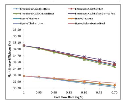
The trends for plant energy efficiency are similar as those observed for the boiler energy efficiency. In case of a fixed fuel flow rate, the plant energy efficiency decreases from 35.02% to 34.65%, 34.66%, 34.61%, and 34.69% for blends of bituminous coal/rice husk, bituminous coal/sawdust, bituminous coal/chicken litter, and bituminous coal/refuse derived fuel respectively, when the co-firing ratio increase from 0% to 30%. Similarly, the plant energy efficiency decreases from 34.08% for the
