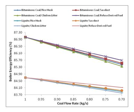
The overall plant energy efficiency also decreases as the biomass proportion increases, as is shown in Figures 5 and 6.
