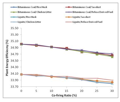
Figure 5. Effect of co-firing on plant energy efficiency based on a fixed fuel flow rate.
