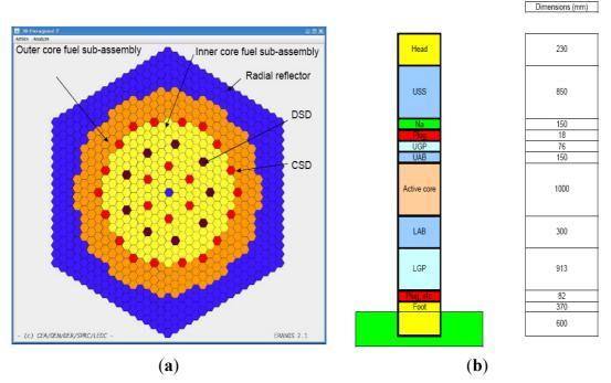
Two figures of merit are considered: the core sodium void reactivity effect (SVRE) and the extended SVRE. The SVRE refers to the voiding of the total active height for the inner and outer fuel zone and the extended SVRE refers, in addition to the active height, to the voiding in the above structures (UGP, UAB, plugs and Na plenum regions). For both figures only voiding inside the wrapper is considered (*i.e.*, sodium between SAs is not removed).
