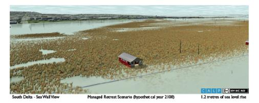
**Figure 16.** Managed Retreat Scenario, Ladner, Aerial View. The Managed Retreat scenario maintains, strengthens, and raises Delta's dike and seawall infrastructure around Ladner [37].
