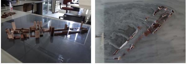
The most important results of the experiment are to show the transversal flows that could to be blocked by dense construction in the east side of the street. The city sector behind the street needs the air flow to guarantee heat evacuation and air change possibility using natural ventilation design strategies.
