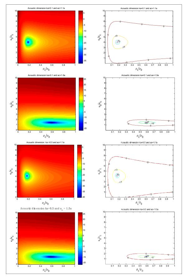
**Figure 3.** SCS variation (dB) obtained by varying the density and bulk modulus of the coating in the plasmonic scattering region.  $k_0a$  and  $a_c$  values are indicated in each panel.
