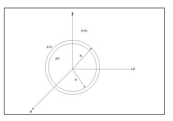
Figure 1. Geometry of the problem: the coated sphere.
