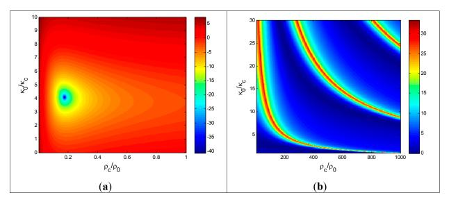
We therefore focus on the plasmonic scattering region and analyze the sensitivity of the SCS to parameter variations for different coating thicknesses ( $a_c = 1.1a$  and 1.5a) and sphere dimensions ( $k_0a = 0.1$ , 0.5 and 1.0). All of these cases satisfy the condition of object smaller than the wavelength of the impinging wave.
