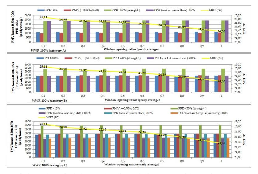
**Figure 11.** Predicted Mean Vote (PMV) and Predicted Percentage of Dissatisfied People (PPD) for categories A,B, and C by means of hours (out of 8760 h in a whole year) for WWR 100% with all window opening ratios (from 0.1 to 1) with M: 1.2 met, air speed of 0.15–0.3 m/s, clothing value with 0.6–0.95 clo.
