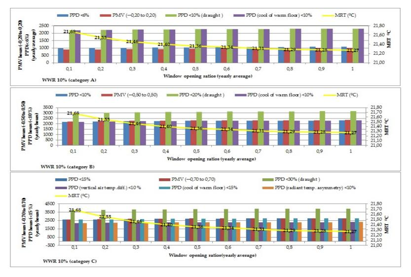
**Figure 2.** Predicted Mean Vote (PMV) and Predicted Percentage of Dissatisfied People (PPD) for categories A,B, and C by means of hours (out of 8760 h in a whole year) for WWR 10% with all window opening ratios (from 0.1 to 1) with M: 1.2 met, air speed of 0.15–0.3 m/s, clothing value with 0.6–0.95 clo.
