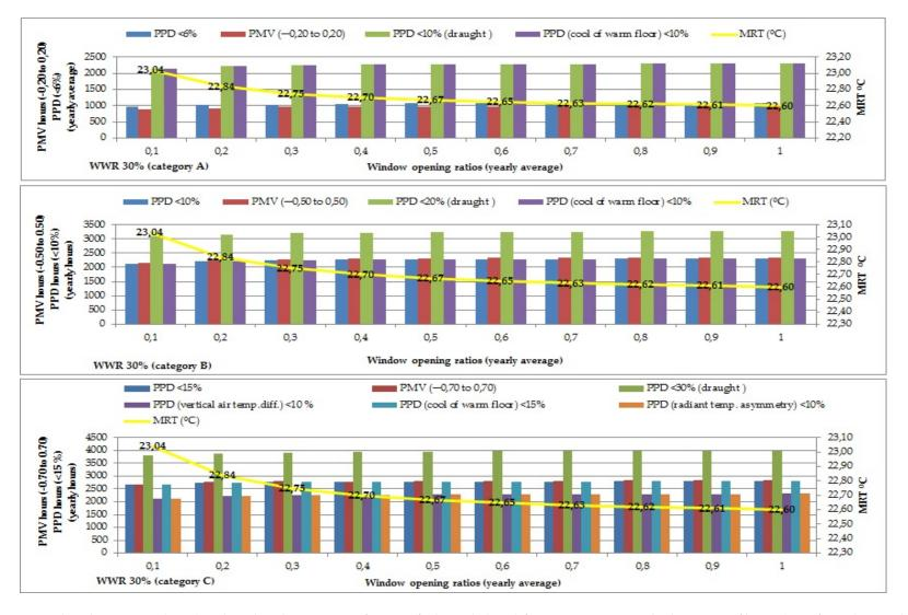
**Figure 4.** Predicted Mean Vote (PMV) and Predicted Percentage of Dissatisfied People (PPD) for categories A,B, and C by means of hours (out of 8760 h in a whole year) for WWR 30% with all window opening ratios (from 0.1 to 1) with M: 1.2 met, air speed of 0.15–0.3 m/s, clothing value with 0.6–0.95 clo.
