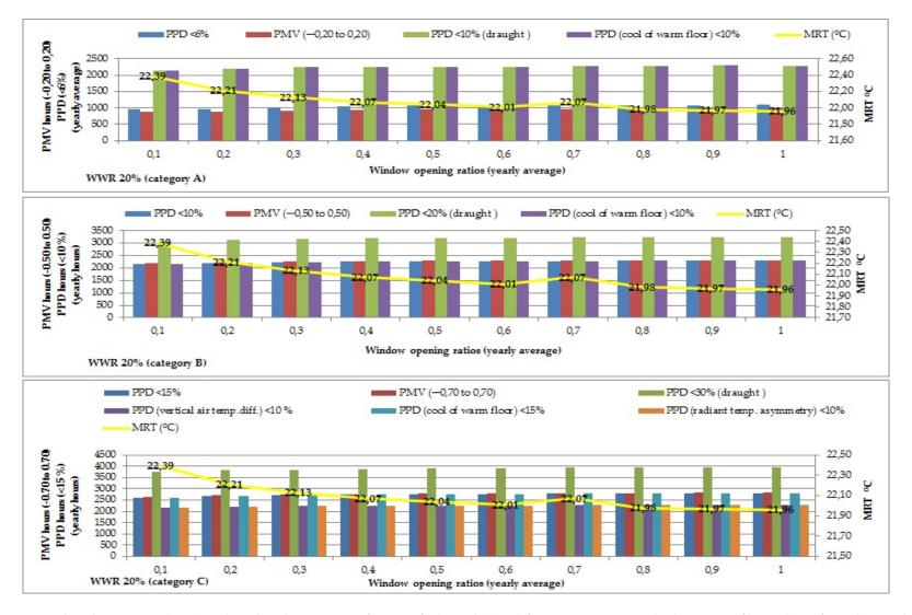
**Figure 3.** Predicted Mean Vote (PMV) and Predicted Percentage of Dissatisfied People (PPD) for categories A,B, and C by means of hours (out of 8760 h in a whole year) for WWR 20% with all window opening ratios (from 0.1 to 1) with M: 1.2 met, air speed of 0.15–0.3 m/s, clothing value with 0.6–0.95 clo.
