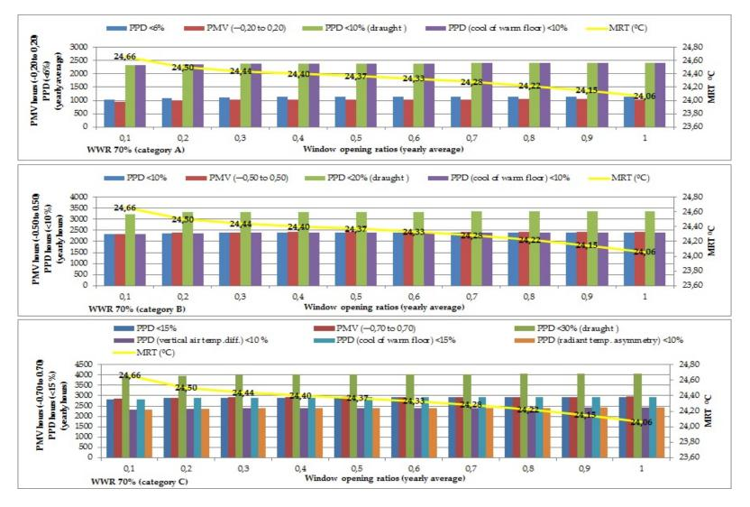
**Figure 8.** Predicted Mean Vote (PMV) and Predicted Percentage of Dissatisfied People (PPD) for categories A,B, and C by means of hours (out of 8760 h in a whole year) for WWR 70% with all window opening ratios (from 0.1 to 1) with M: 1.2 met, air speed of 0.15–0.3 m/s, clothing value with 0.6–0.95 clo.
