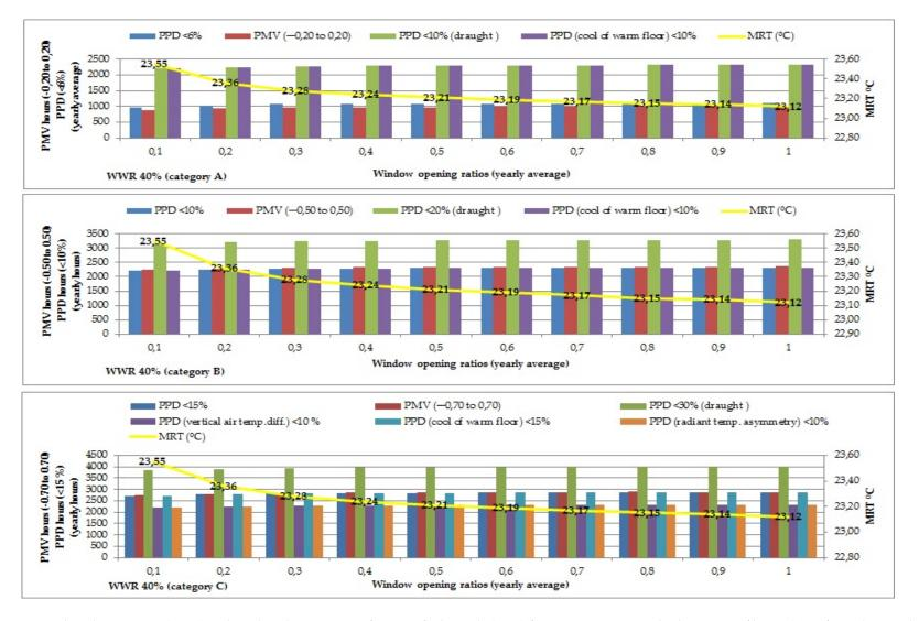
**Figure 5.** Predicted Mean Vote (PMV) and Predicted Percentage of Dissatisfied People (PPD) for categories A,B, and C by means of hours (out of 8760 h in a whole year) for WWR 40% with all window opening ratios (from 0.1 to 1) with M: 1.2 met, air speed of 0.15–0.3 m/s, clothing value with 0.6–0.95 clo.
