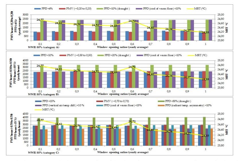
**Figure 9.** Predicted Mean Vote (PMV) and Predicted Percentage of Dissatisfied People (PPD) for categories A,B, and C by means of hours (out of 8760 h in a whole year) for WWR 80% with all window opening ratios (from 0.1 to 1) with M: 1.2 met, air speed of 0.15–0.3 m/s, clothing value with 0.6–0.95 clo.
