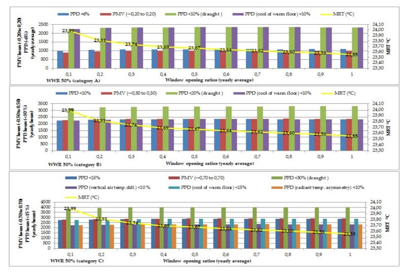
**Figure 6.** Predicted Mean Vote (PMV) and Predicted Percentage of Dissatisfied People (PPD) for categories A,B, and C by means of hours (out of 8760 h in a whole year) for WWR 50% with all window opening ratios (from 0.1 to 1) with M: 1.2 met, air speed of 0.15–0.3 m/s, clothing value with 0.6–0.95 clo.
