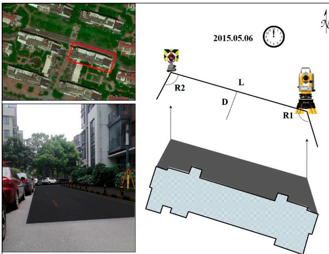
Figure 2. Measurement location and method.
