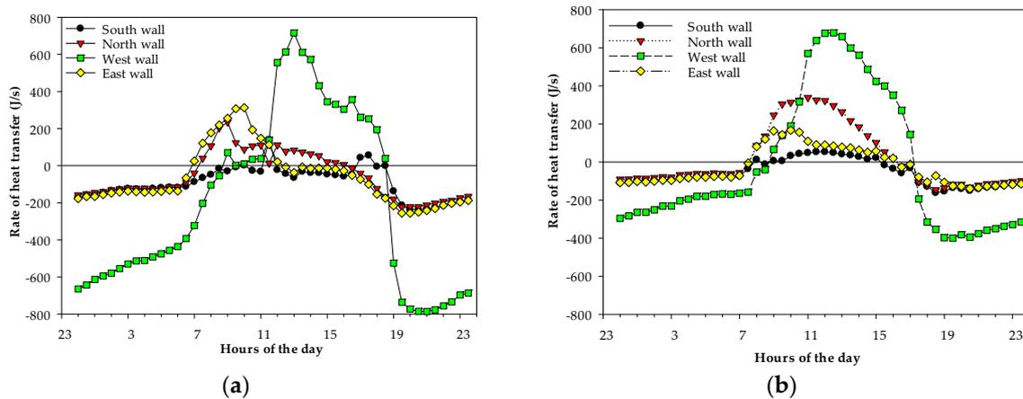
**Figure 8.** (a) Summer season rate heat transfer through perimeter walls; and (b) winter season rate heat transfer through perimeter walls.
