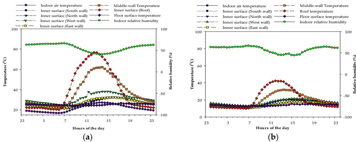
**Figure 7.** (a) Average summer daily indoor temperature and relative humidity response to the components of thermal envelope surface temperature; and (b) average winter daily indoor temperature and relative humidity response to the components of thermal envelope surface temperature.
