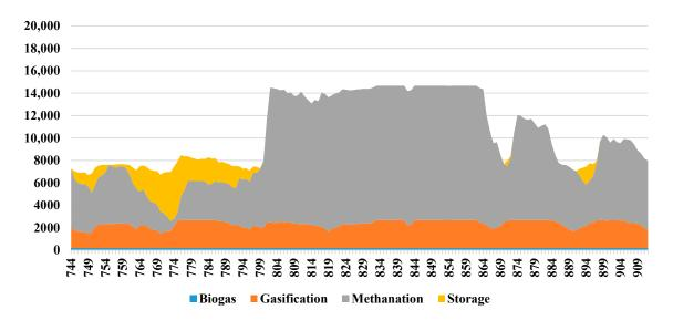
**Figure S5.** Grid gas supply (MW<sub>gas</sub>): February 1-7. Production of PtG methane is high during periods of high wind production during the study week. PtG production as occurs during noon solar PV production peaks. Gasified biomass also contributes to the gas grid during winter months.
