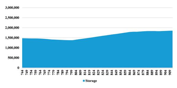
**Figure S6.** Grid gas storage (MWh<sub>gas</sub>): February 1-7. Maximum storage is 3 800 000 MWh<sub>gas</sub>. Storage levels of grid gas slightly increase during one of the weeks of highest gas demand due to high levels of PtG production that resulted from relatively high wind power production.
