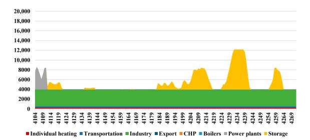
**Figure S10.** Grid gas demand (MW<sub>gas</sub>): June 20-26. Demand for grid gas is relatively low during the study period. Excess gas is allocated to storage.
