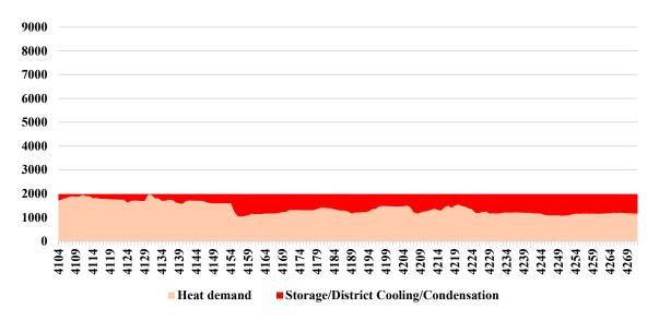
**Figure S7.** DH demand (MW<sup>th</sup>): June 20-26. Heat demand is low during the summer months. This study period also represents a time of reduced industrial heat use due to summer holidays. A significant amount of excess heat is therefore condensed.
