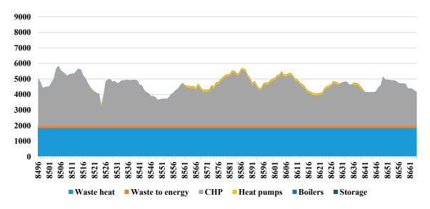
**Figure S14.** DH supply (MWth): December 20-26. CHP plants run at close to maximum capacity during this period. Colder temperatures during the mid-week necessitate the use of heat pumps for the DH system.
