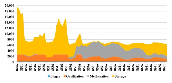
**Figure S17.** Grid gas supply (MW<sub>gas</sub>): December 20-26. High grid gas demand is mostly provided by storage over the study period. Relatively high PtG methane production is utilized directly after midweek. Biomass gasification is relatively strong during this period of high gas demand.
