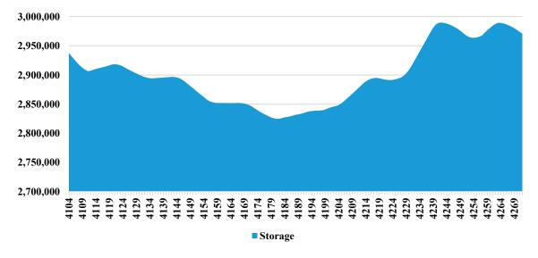
**Figure S12.** Grid gas storage (MWh<sub>gas</sub>): June 20-26. Maximum storage is 3 800 000 MWh<sub>gas</sub>. Small, daily increases in grid gas storage correspond to peaks in solar PV production. Small amounts of gas are used during the evening hours to produce power in CHP plants. Grid gas storage is close to maximum during the study period.
