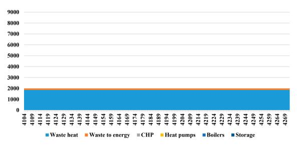
**Figure S8.** DH supply (MWth): June 20-26. Supply of heat mostly comes from waste heat resulting from the PtG process.
