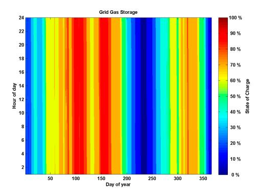
**Figure 4.** State of charge of grid gas storage. The grid gas storage is used as a seasonal balancing component for the energy system, as documented by the seasonal charging and discharging pattern.
