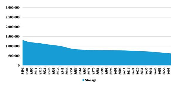
**Figure S18.** Grid gas storage (MWh<sub>gas</sub>): December 20-26. Maximum storage is 3 800 000 MWh<sub>gas</sub>. Grid gas storage is at relatively low levels for the year due to high demand. Storage levels decrease smoothly, however, due to variable production of synthetic methane from gasification of biomass and PtG.
