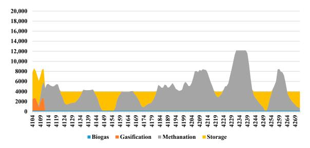
**Figure S11.** Grid gas supply (MW<sub>gas</sub>): June 20-26. PtG methane production corresponds to peaks in solar PV production during the study period. Gasification of biomass is unnecessary during most of the study period.
