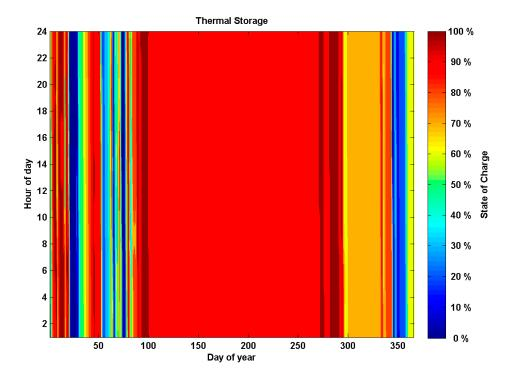
**Figure 3.** State of charge of DH storage. Finland currently has high levels of thermal energy storage associated with the DH system. Much of it is unused during the summer months, but it has an important function during the winter.
