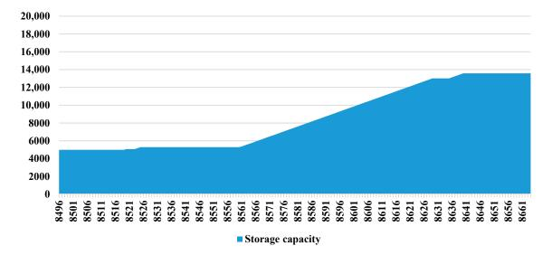
**Figure S15.** DH storage (MWhth): December 20-26. Maximum storage is 20 000 MWhth. Thermal storage approaches its lowest levels for the year during the study period due to relatively high demand. High demand for electricity during a windy and cold period in the middle of the study period results in high CHP production. This is also a time of high electricity demand during Christmas. Heat storage levels moderately increase as a result of excess heat production during the daytime.
