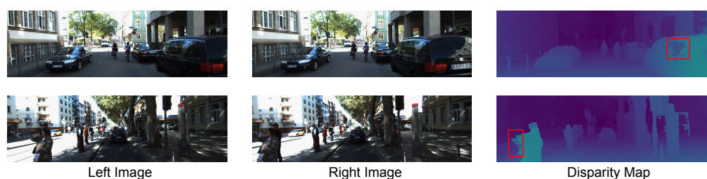
Figure 7. Failure examples. Our network still cannot deal with specular reflection and object occlusion well.
