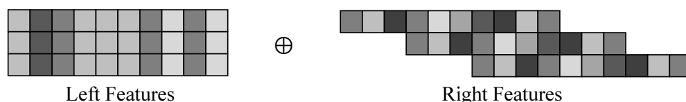
Figure 3. Our sparse cost volume ( S = 3 ). We propose a parameter S for stride size to control the redundancy.
