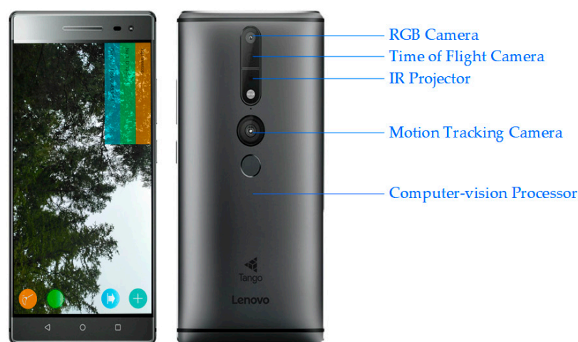
Figure 2. Structure of a smart phone (Lenovo Phab 2 Pro) with RGB-D SLAM.
