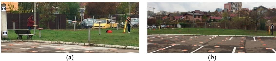
**Figure 5.** (a) Taking the measurements using a miniprism and (b) two Leica TCR 405 total stations, centered on A and B GNSS points.
