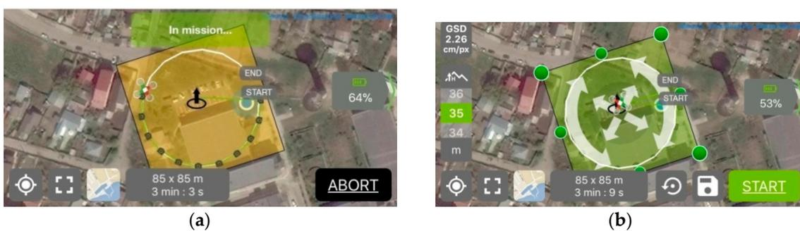
**Figure 6.** Screen shots during the UAS image acquisition over the 3D calibration field for digital cameras mounted on UAS platforms at (a) 28 m height and (b) 35 m height.
