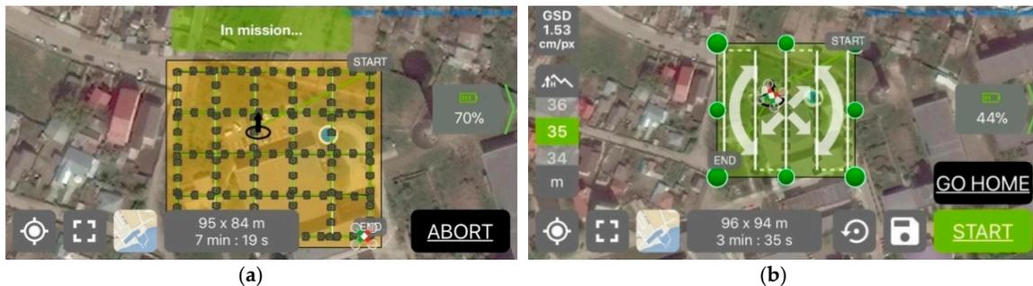
Figure 14. Taking the UAS images over the calibration field at (a) 28 m and (b) 35 m.
