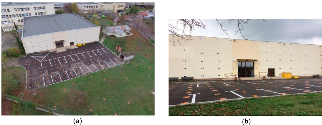
**Figure 2.** (a) UAS image over the 3D calibration field of digital non-metric cameras mounted on Unmanned Aerial Systems, (b) ground image.
