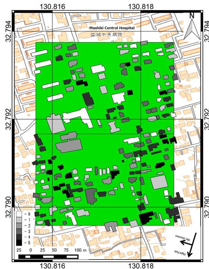
**Figure 3.** Distribution of the damaged buildings in a sampled region of Mashikimachi town.
