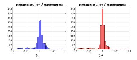
**Figure 3.** Comparisons of total variation  $TV-L^2$  and  $TV-L^1$  destriping for the results shown in Figure 1. (a) Histogram of function *G* for  $TV-L^2$  reconstruction. (b) Histogram of function *G* for  $TV-L^1$  reconstruction.  $TV-L^1$  reconstruction is pointier than  $TV-L^2$  reconstruction. It is also centered at 1, as opposed to  $TV-L^2$  reconstruction, which further indicates better accuracy of  $TV-L^1$  model.
