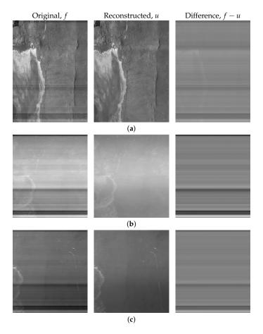
**Figure 7.** Images with stripes captured by Airborne Multi-angle Spectro Polarimetric Imager (AirMSPI) instrument at Mojave, California (**left**); destriped images using total variation  $TV-L^1$  model (**center**); and differences between captured and destriped images (**right**) are shown. The bands and viewing angles are (**a**) 380 nm band at nadir angle, (**b**) 355 nm band at 66.1°F angle, and (**c**) 355 nm band at 66.1°A angle; 355 nm band at nadir angle is shown in Figure 1.
