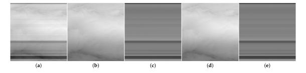
**Figure 4.** (a) The 355 nm channel image with stripes depicting clouds over the Pacific Ocean captured by Airborne Multi-angle Spectro Polarimetric Imager (AirMSPI) instrument from  $66.0^{\circ}$ F angle. (b) Destriped image using total variation TV– $L^2$  model. (c) Difference between captured image from (a) and TV– $L^2$  destriped image from (b). (d) Destriped image using TV– $L^1$  model. (e) Difference between captured image from (a) and TV– $L^1$  destriped image from (d).
