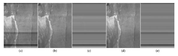
**Figure 1.** (a) The 355 nm channel image with stripes captured by Airborne Multi-angle Spectro Polarimetric Imager (AirMSPI) instrument from nadir angle at Mojave, California. (b) Destriped image using total variation  $TV-L^2$  model. (c) Difference between captured image from (a) and  $TV-L^2$  destriped image from (b). (d) Destriped image using  $TV-L^1$  model. (e) Difference between captured image from (a) and  $TV-L^1$  destriped image from (d).
