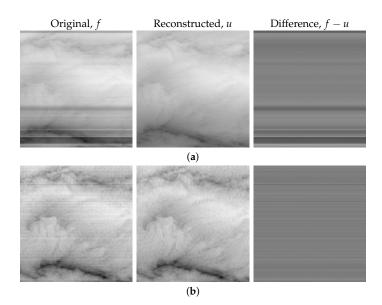
**Figure 8.** Images with stripes depicting clouds over the Pacific Ocean captured by Airborne Multi-angle Spectro Polarimetric Imager (AirMSPI) instrument (**left**), destriped images using total variation  $TV-L^1$  model (**center**), and differences between captured and destriped images (**right**) are shown. The bands are (**a**) 380 nm, and (**b**) 660 nm, all at 66.0°F; 355 nm band at 66.0°F angle is shown in Figure 4.
