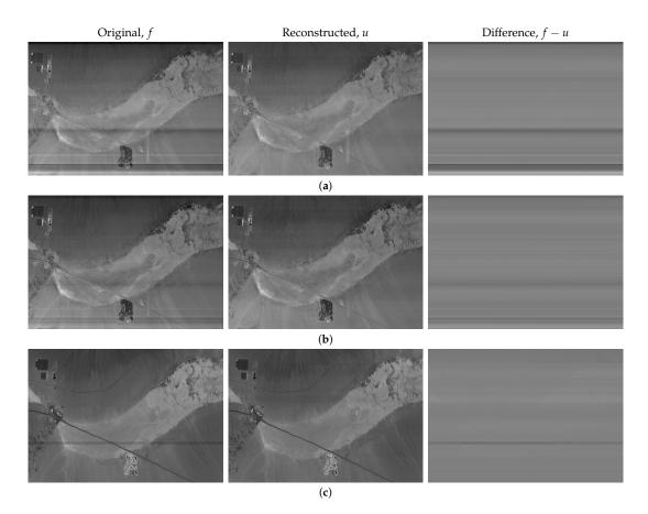
**Figure 9.** Images with stripes of dry Ivanpah Lake, California, captured by Airborne Multi-angle Spectro Polarimetric Imager (AirMSPI) instrument (**left**); destriped images using total variation  $TV-L^1$  model (**center**); and differences between captured and destriped images (**right**) are shown. The bands are (**a**) 355 nm, (**b**) 380 nm, and (**c**) 865 nm, all at nadir angle.
