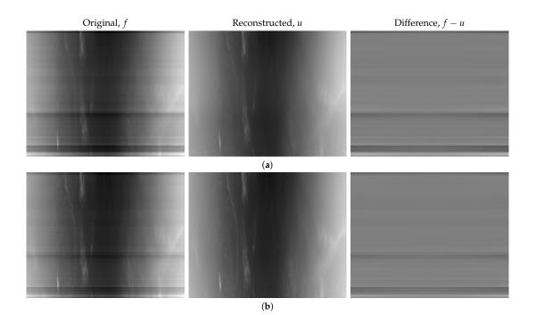
**Figure 10.** Images captured by Airborne Multi-angle Spectro Polarimetric Imager (AirMSPI) instrument at Avalon, California (**left**); destriped images using total variation  $TV-L^1$  model (**center**); and differences between captured and destriped images (**right**) are shown. The bands are (**a**) 355 nm, and (**b**) 380 nm, both captured using the continuous-sweep observing mode.
