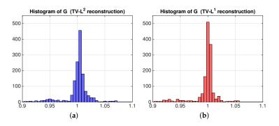
**Figure 6.** Comparisons of total variation  $TV-L^2$  and  $TV-L^1$  destriping for the results shown in Figure 4. (a) Histogram of function *G* for  $TV-L^2$  reconstruction. (b) Histogram of function *G* for  $TV-L^1$  reconstruction.  $TV-L^1$  reconstruction. It is also centered at 1, as opposed to  $TV-L^2$  reconstruction, which further indicates better accuracy of  $TV-L^1$  model.
