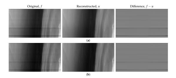
**Figure 11.** Images with stripes captured by Airborne Multi-angle Spectro Polarimetric Imager (AirMSPI) instrument at Fallbrook, California (**left**); destriped images using total variation  $TV-L^1$  model (**center**); and differences between captured and destriped images (**right**) are shown. The bands are (**a**) 355 nm, and (**b**) 380 nm, both captured using the continuous-sweep observing mode.
