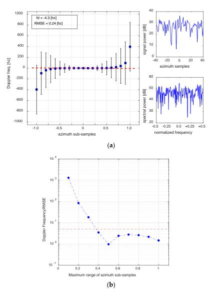
**Figure 3.** An application result for a weak stationary target, to determine an optimum ratio of Doppler frequency to RMSE for estimation on land. The PSLR of the target is -4.3 dB, with an SCR of 9.6 dB. A ratio of larger than 5–10 would be acceptable for the on-land point targets.
