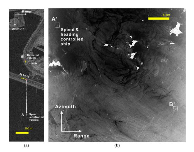
**Figure 1.** Two synthetic aperture radar (SAR) images used in this study: (**a**) TerraSAR-X SLC image, in which a speed-controlled vehicle A is observed. (**b**) KOMPSAT-5 SLC image over coastal areas, in which a speed and heading controlled ship A' for the experiment, as well as numerous high velocity ships, are observed.
