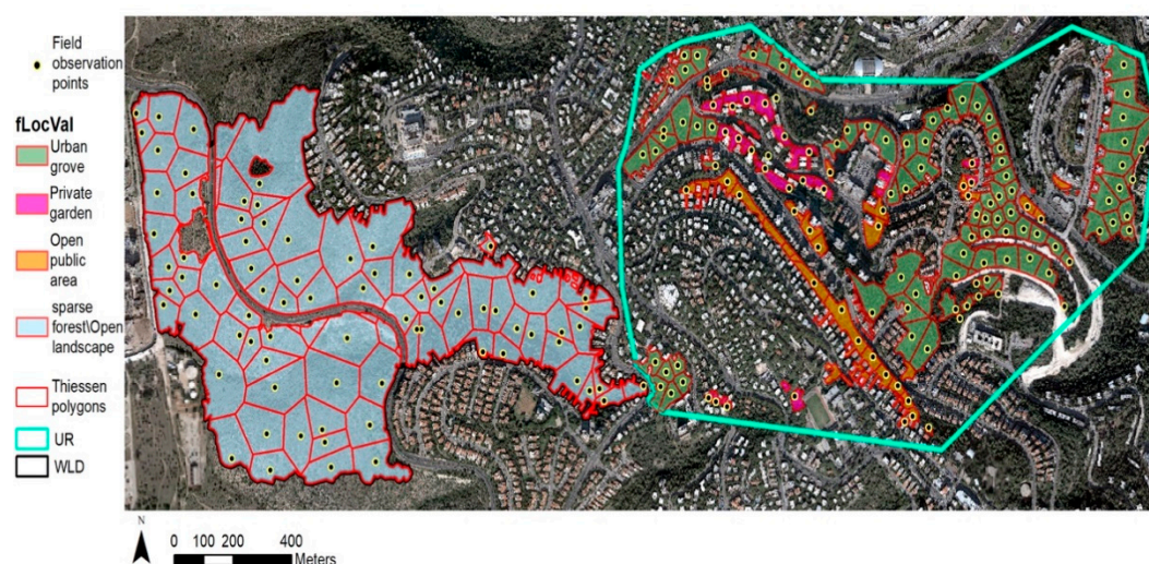
Figure A2. The 212 Thiessen polygons in the WUI burnt area used to map the environmental factors used in i-Tree model for the spatially distributed economic loss calculations.
