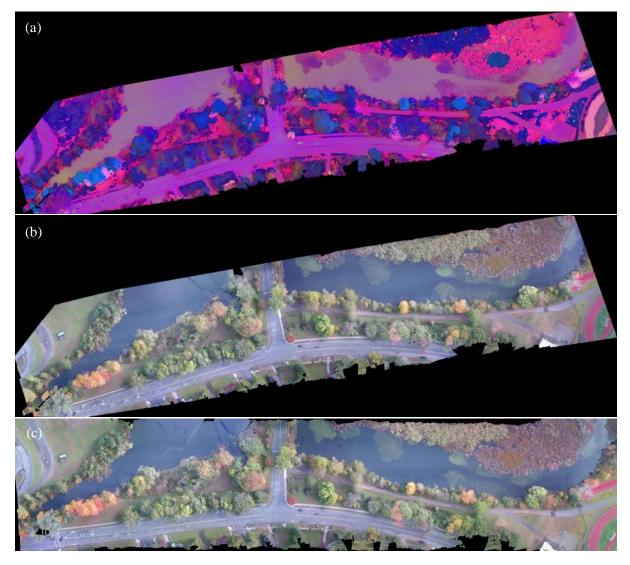
**Figure S3.** Comparison between the HSV-based orthomosaic and the original RGB-based orthomosiac: (a) The HSV-based orthomosaic in HSV color. (b) The HSV-based orthomosaic converted to its corresponding RGB colormap. (c) The original RGB-based orthomosaic (Figure 4a).
