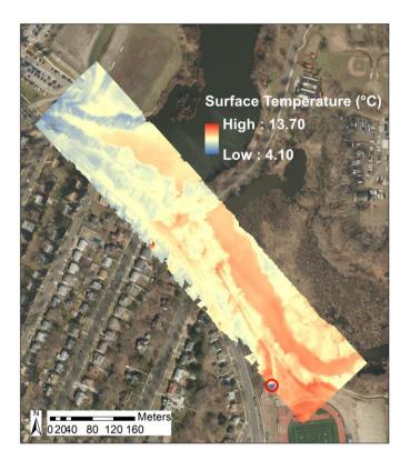
**Figure S1.** The temperature map in degree Celsius converted from the DN value in the thermal othomosaic (Figure 6b) by the regression equation (Figure 10b). The red circle indicates a spot with an extremely low temperature (-6.7 °C) due to the low-emissivity of a metal roof on a garage.
