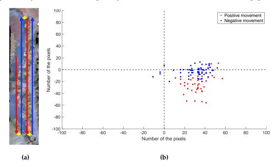
**Figure S2.** The misalignment caused by shutter delay for different moving directions. (a) The RGB orthomosaic with the flying route marked by arrows. The positive movement is indicated by red arrows and the negative movement by blue arrows. (b) Scatter plot of misalignment in two dimensions. Red dots indicate positive UVA movement and blue dots indicate negative movement.
