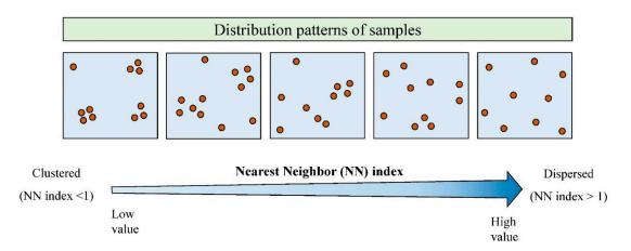
**Figure 2.** Schematic diagram of the relationship between the distribution pattern of samples and the nearest neighbor (NN) index.
