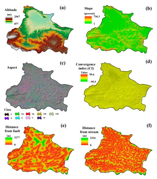
**Figure 7.** Groundwater-affecting factors (GAFs) in the study area: (**a**) altitude, (**b**) slope, (**c**) aspect, (**d**) convergence index, (**e**) distance from fault, and (**f**) distance from stream (for a detailed description of lithological classes, see Table 3).
