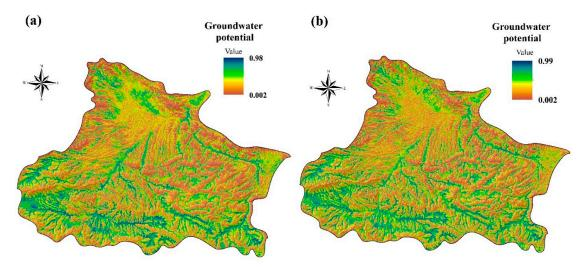
**Figure 9.** Groundwater potential maps of the study area produced using the random forest (RF) model and based on: (a) the simple random method, and (b) the selection of absence samples (SAS) method.
