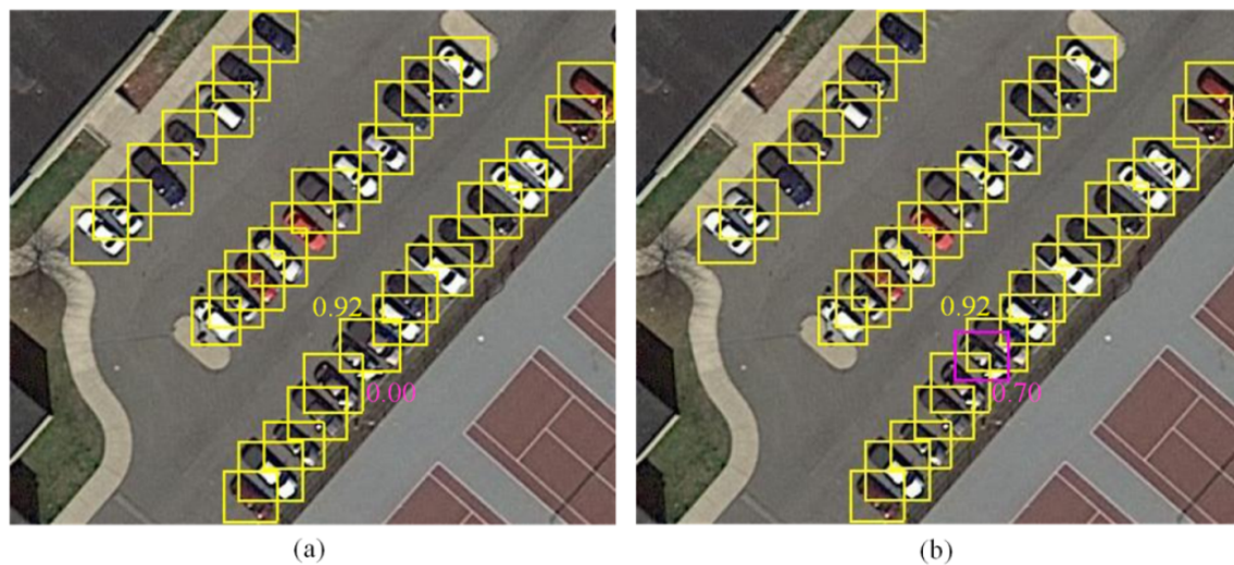
Figure 8. Effect of the Soft-non-maximum suppression (NMS). In (a), a car cannot be detected because its confidence is set to 0 by NMS due to its Intersection-over-Union (IOU) with the nearest car, having a higher confidence 0.92, more than a thresh; however, in (b), the confidence of the car not detected in (a) is set to 0.70 instead of 0 according to Equation (13).
