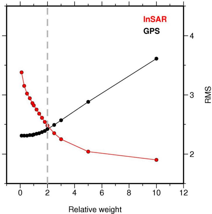
**Figure 4.** Relationship between RMS (in mm) data reduction and relative weighting factors. The black circles represent the RMS of the GPS datasets, while the red ones are relevant to the InSAR measurements. The gray dashed line represents our choice of weighting factor.
