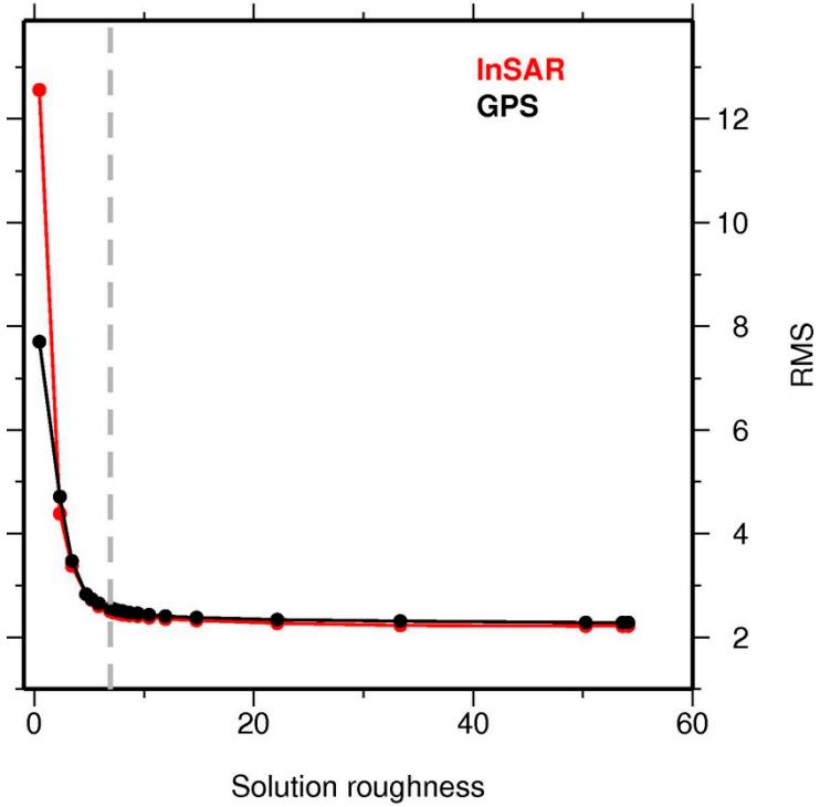
**Figure 3.** Trade-off curves between RMS (in mm) data and model roughness. The black circles represent the RMS of the GPS datasets, while the red ones are relevant to the InSAR measurements. The gray dashed line represents our choice of smoothing factor.
