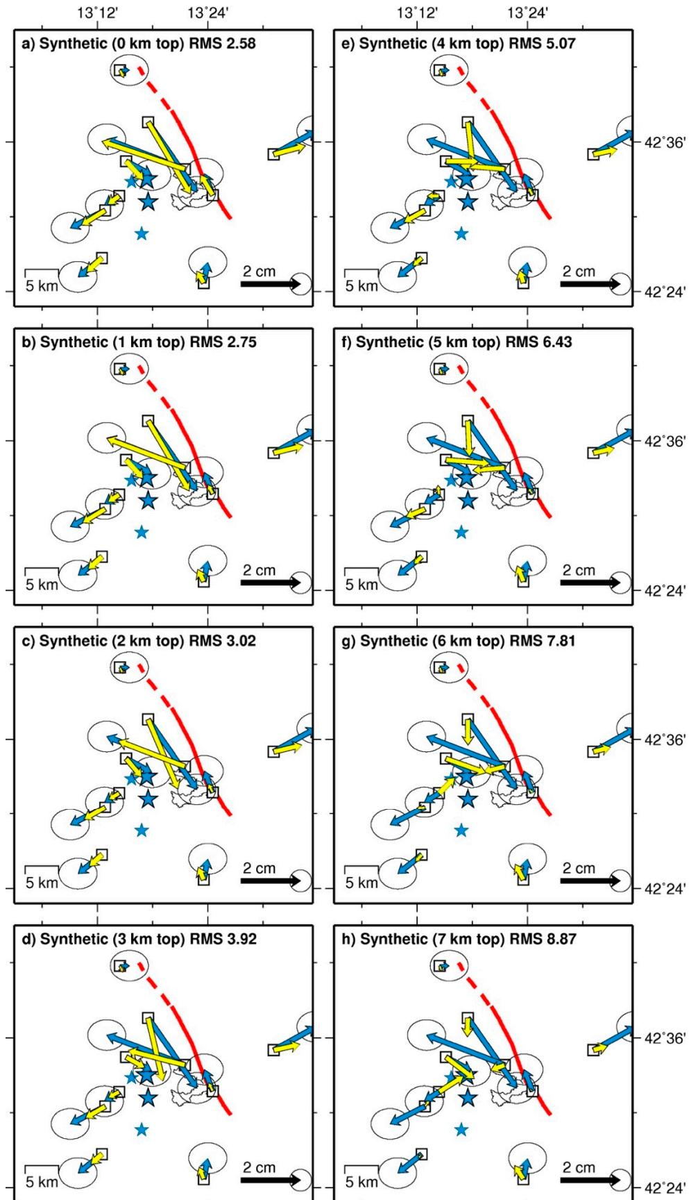
**Figure 5.** Fit to the horizontal components of GPS data as a function of the assumed fault top depth. Observed (blue) and modelled (yellow) cumulative GPS displacements: (a) horizontal, and (b) vertical displacements, respectively. Note that increasing the depth of the fault, significantly worsens the fit to the data. .
