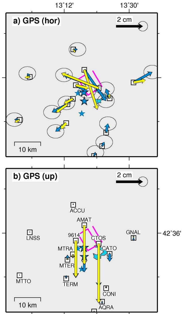
**Figure 2.** Observed (blue) and modelled (yellow) cumulative GPS displacements: (a) horizontal, and (b) vertical displacements, respectively. The blue stars are the four largest events of the 2017 seismic sequence. The violet box represents our best-fit uniform-slip solution.
