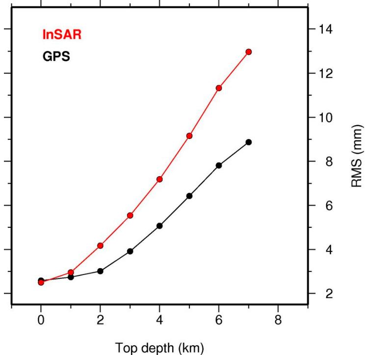
**Figure 7.** Trade-off curves between RMS (in mm) data reduction and assumed fault top depth. The black circles represent the RMS of the GPS datasets, while the red ones are relevant to the InSAR measurements. Note that increasing the depth of the fault, significantly worsens the fit to the data.
