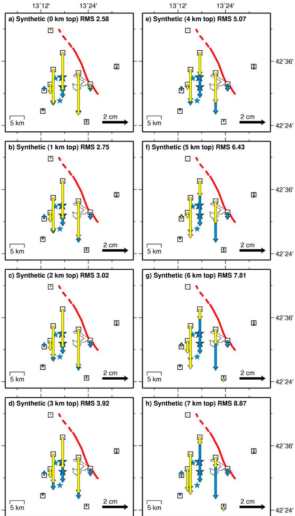
**Figure 6.** Fit to the vertical component of GPS data as a function of the assumed fault top depth. Observed (blue) and modelled (yellow) cumulative GPS displacements: (a) horizontal, and (b) vertical displacements, respectively. Note that increasing the depth of the fault, significantly worsens the fit to the data.
