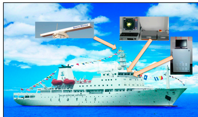
Figure 5. Installation of the ship-borne radar oil spill data acquisition system onboard the Yukun [26].
