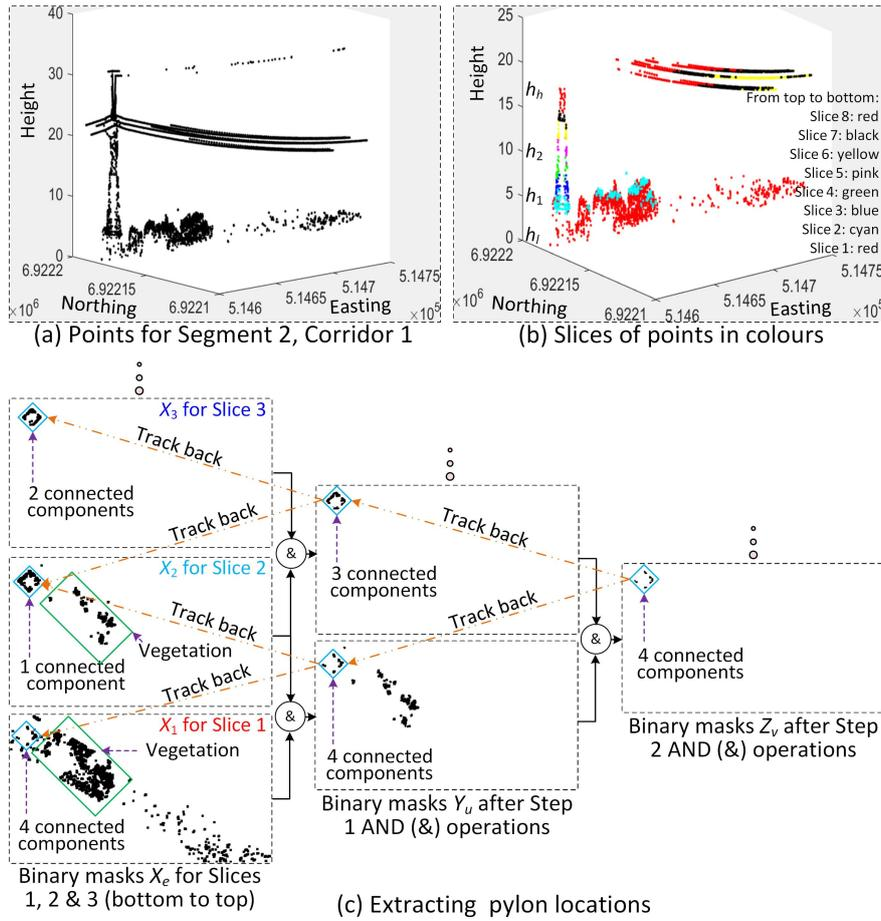
**Figure 7.** Extraction of pylon locations. Easting, Northing and Height are in metres (m). Within the binary images in (c), black pixels indicate “true” and white pixels indicate “false” for any non-ground objects (i.e., pylon, tree, etc.).
