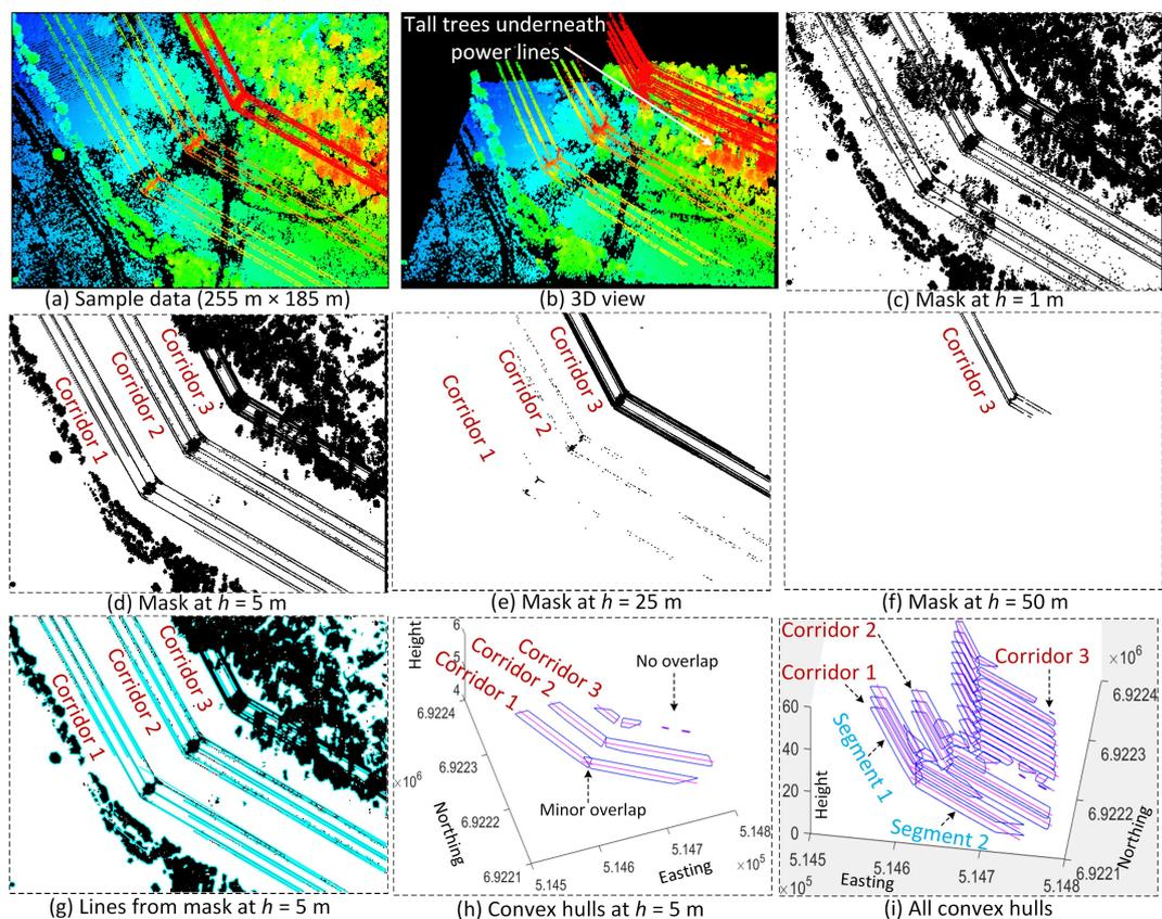
Figure 2. Sample input data and PL masks  $M_h$  at different height levels  $h$ .
