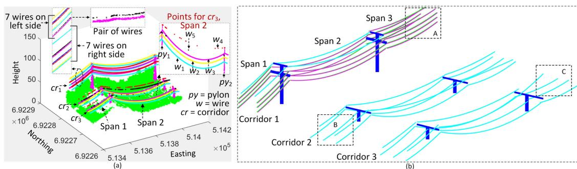
**Figure 15.** (a) Ground truth data for Site 3 (see Figure 14); and (b) extracted wires from an extended area of Site 3.
