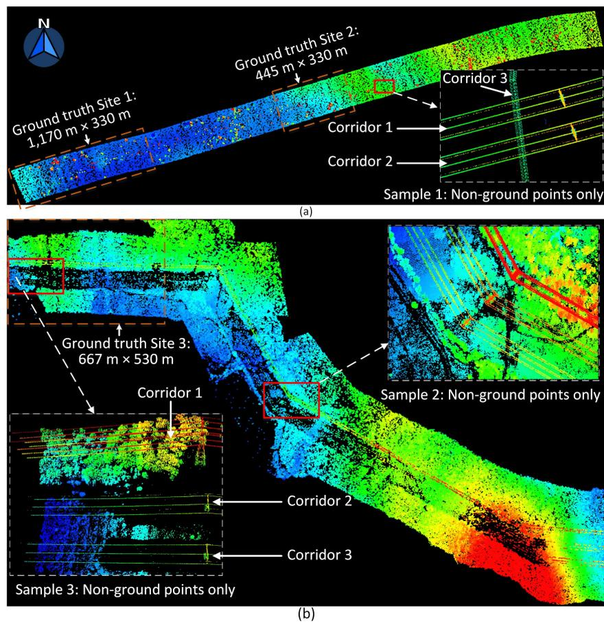
**Figure 14.** The test datasets: (a) Maindample, Victoria; and (b) Bindebango, Queensland. In the three samples, only the non-ground points with at least 1 m height above the ground are shown. Samples 2 and 3 are used in Figures 2 and 12, respectively.
