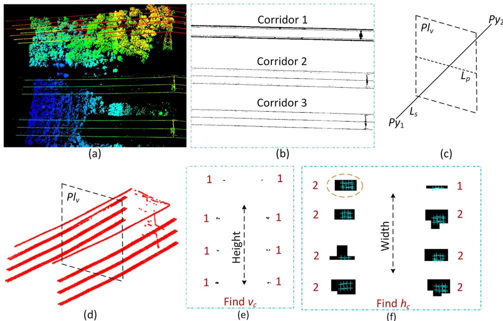
**Figure 12.** Counting the number of wires: (a) sample scene; (b) PL mask  $M_p$ ; (c) corridor axis  $L_s$  and vertical plane  $Pl_v$ ; (d) input points between an end and a pylon of Corridor 1; (e) clusters of wires in vertical mask  $M_v$ ; and (f) connected components from PL mask  $M_p$  ( $L_p$  = perpendicular line to  $L_s$ ,  $v_c$  = vertical count of wires and  $h_c$  = horizontal count of wires).
