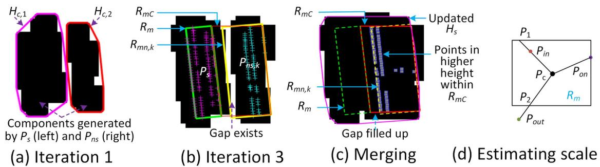
**Figure 10.** Binary masks of points in slices during pylon extraction: (a–c) Within the binary images, black pixels indicate “true” and white pixels indicate “false” for pylons; and (d) how to estimate scaling factor.
