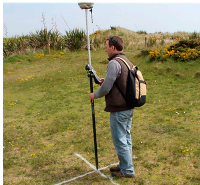
Figure 6. Ground control points (GCPs) set on site for UAS surveying. Photo taken by the author.
