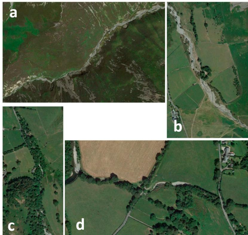
**Figure 2.** Changing character of Liza Beck, (a) bedrock/boulder cascade, (b) boulder dominated torrent, (c) single-thread/bifurcated, (d) historically straightened single-thread.
