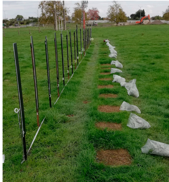
Figure 6. Transect 1 with posts at 0, 1, ..., 8, 10, 11, ..., 20 m. Biomass measured was measured from quadrats at -0.25 to 0.25 m, 0.75 to 1.25 m, ..., 19.75 to 20.25 m.
