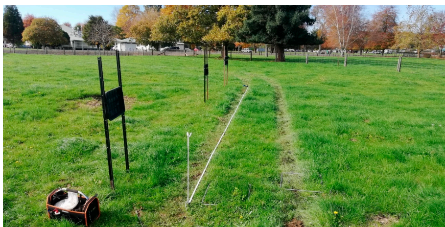
Figure 7. Transect 3 with three 0.5 m-wide reflectors. Ultrasonic profiles and biomass samples were taken from the start of the first post up to the last post. The 0.5\text{ m} \times 0.5\text{ m} quadrat frames can be seen.
