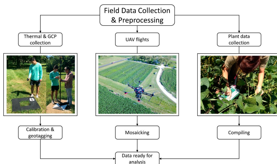
Figure 4. The process for gathering thermal data, UAV imagery, and plant trait data. In the left photo, FLIR TG167 was used to take ground temperature readings over a thermal target, and Trimble Catalyst Differential GPS system was used to record accurate coordinates of ground control targets. In the middle, the UAV system was collecting data over the test site located in Bradford Research Extension Center, Columbia, Missouri. Right photo shows a LI-6400XT Portable Photosynthesis System being used to collect photosynthesis and stomatal conductance.
